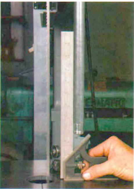
Now check the guidepost. It should be perpendicular to the table. If it's out by \frac{1}{16} in. or more over 6 in. of its height, the saw's performance can be improved by additional adjustments.
