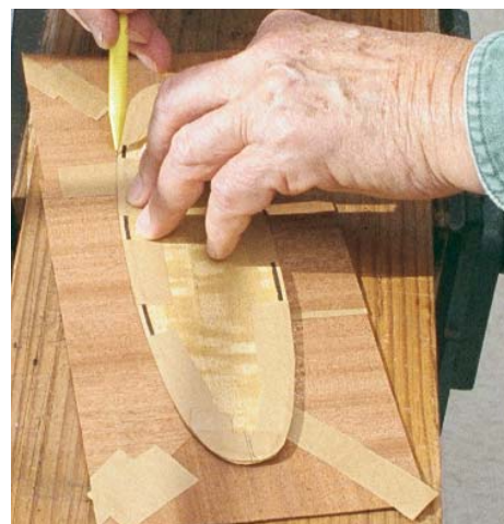
Mark each piece separately. A completed ellipse is used to mark the cutout in the background veneer.
