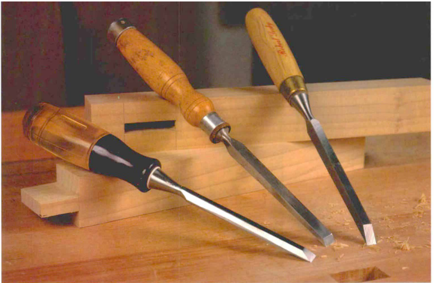
Basic bench chisels—Bevel-edge chisel (left), firmer chisel and mortise chisel all have different tasks in the workshop.
