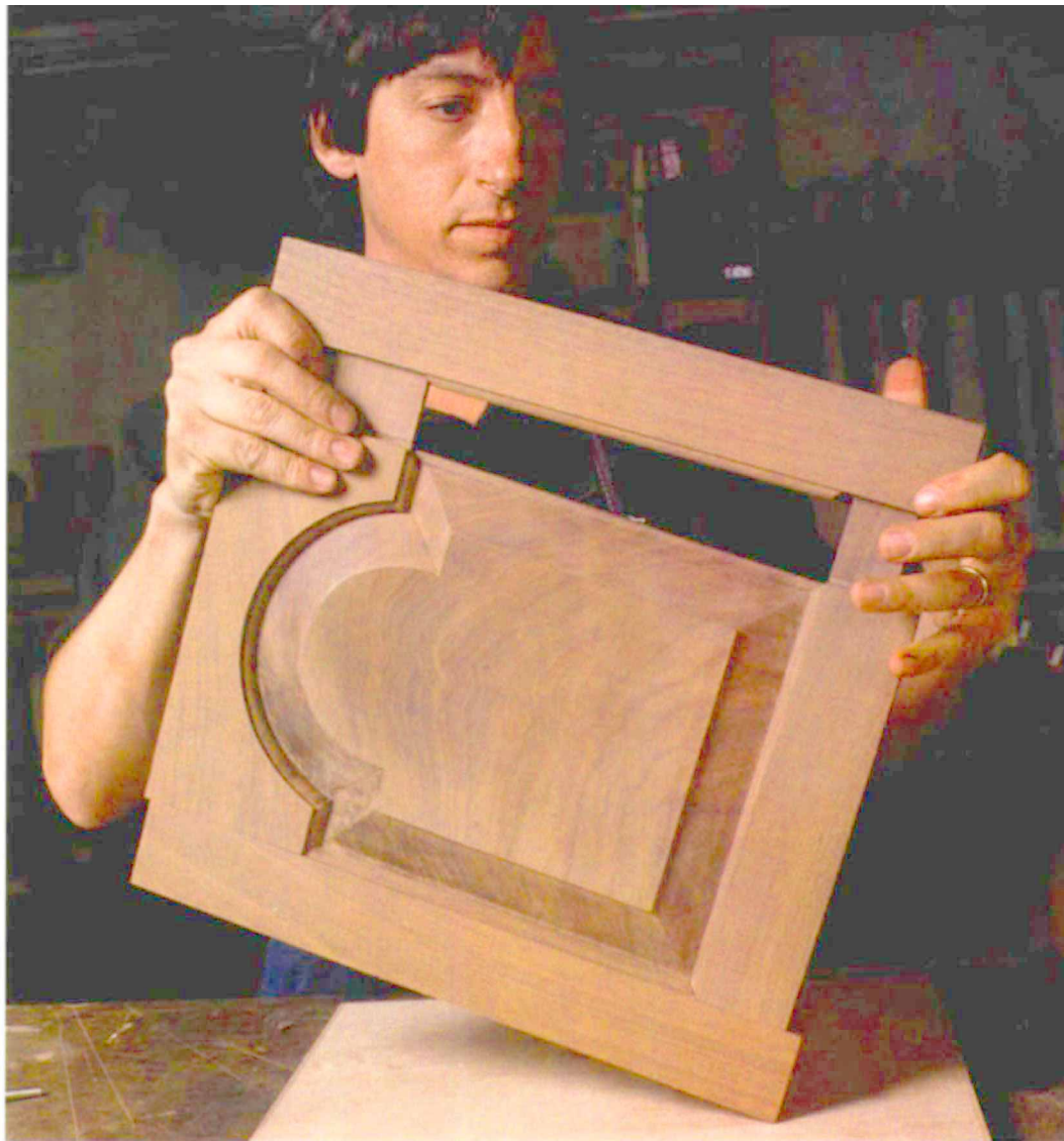
Full-length tenons hold the frame together. The author dry-assembles the completed tombstone door. After glue-up, he trims the door to fit the case opening.
