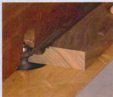
Finish by cutting the bead. Flip molding on its other face; use a \frac{1}{2} -in.-dia. beading bit to shape the edge.
