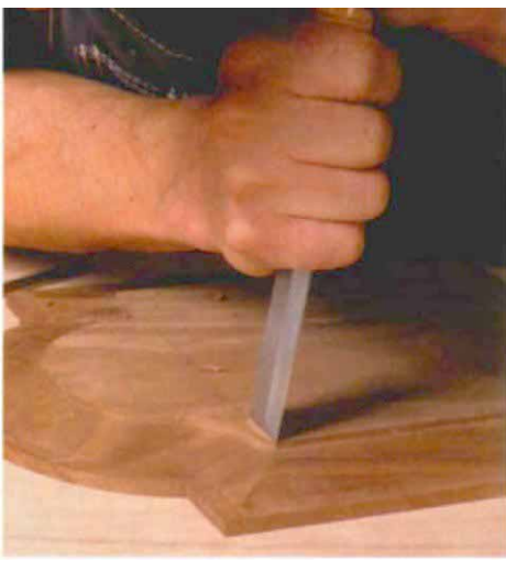
A chisel squares panel corners. A panel-raising router bit leaves corner details unfinished. A chisel cuts the 90° angles at the inside corners.
