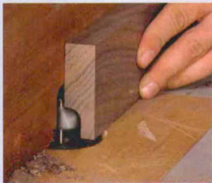
Use a \frac{1}{2} -in.-radius cove bit for first cut. For support, keep the stock for the molding at least 3 in. wide.
