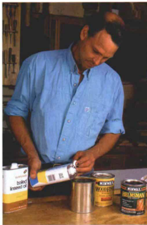
Ingredients are simple; proportions are forgiving. Linseed or tung oil, varnish and turpentine make up the author's favorite finish. A pigment-ed oil stain can be added to give the mixture a little color.
