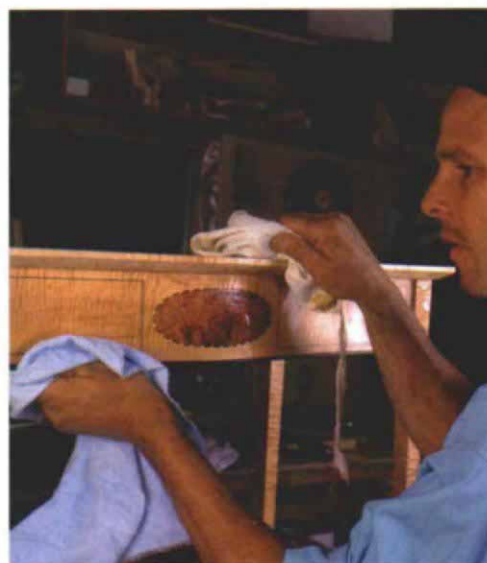
Rub off the excess. Pay close attention to the inside corners and the areas around details like cock beading, where the finish can collect. It's more difficult to remove excess finish after it has hardened.
