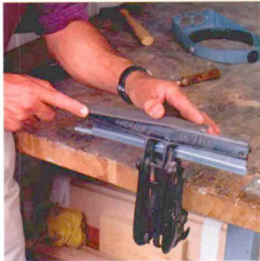
**4. Joint the teeth.** Eliminating teeth and removing the set can create teeth of varying heights. Use a 10-in. mill file to take the tops of the teeth down until they are all at the same height.
