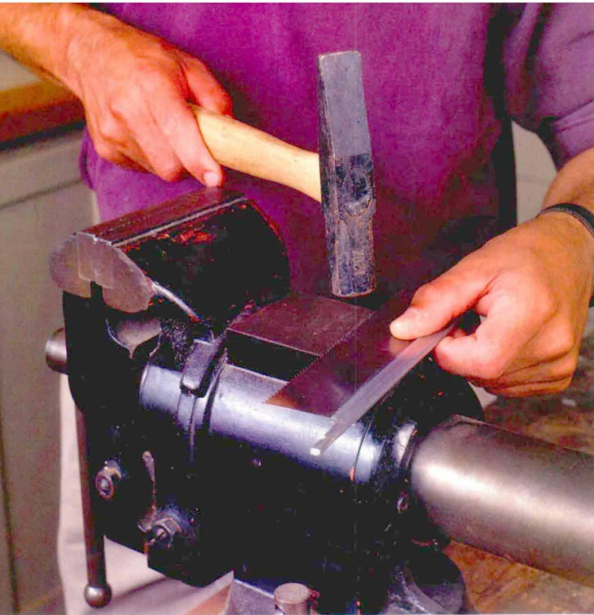
**2. Remove the set.** Put the blade on an anvil or similar surface, and gently hammer out the set. Light taps will do the trick. Remember, you're just flattening a thin sawblade, not working horseshoes.
