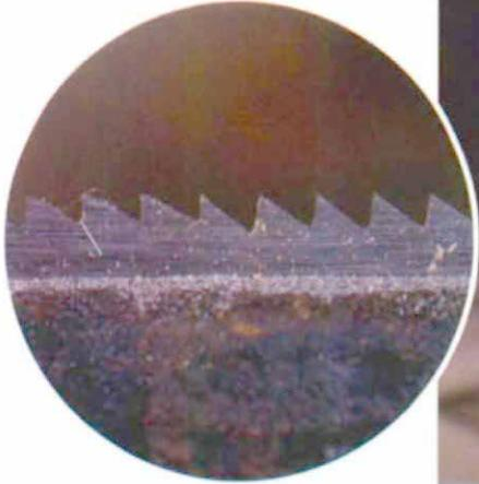
**6. Deburr the teeth.** Filing the teeth will create burrs on the far side of the blade that can cause your saw to catch, drag or wander slightly. To remove these burrs, just pass a coarse stone lightly across the blade.
