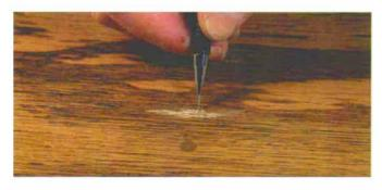
**5.** Scratches give the patch a third dimension. After the first base coat of stain, the author etches grain lines into the surface of the putty repair with a sharp scribe.
