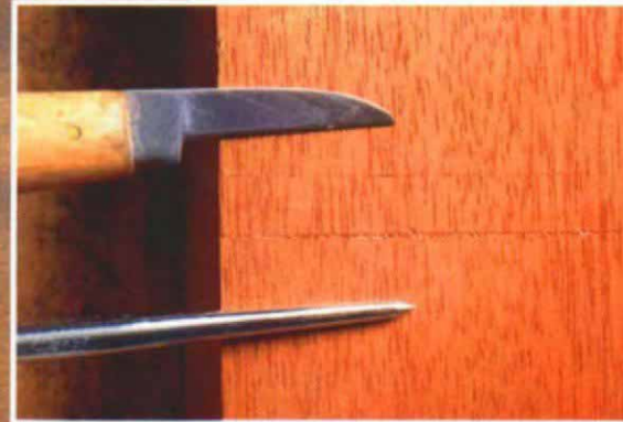
An awl point breaks wood fibers across the grain; a sharp knife cuts them.
