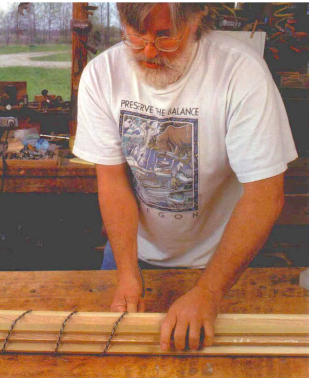
4. Wrap cord tightly around the assembly. Tack the bungee cord at the other end.
