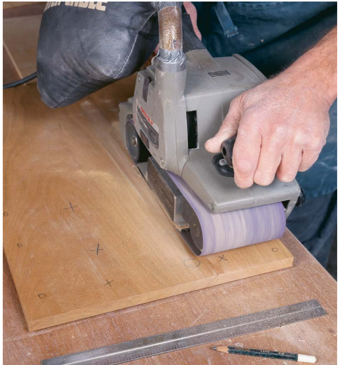
Mark the highs and lows with a soft pencil to indicate which areas need more sanding. The author makes his first pass over the surface of a glued-up cherry panel with high spots marked with X's and low spots marked with O's.
