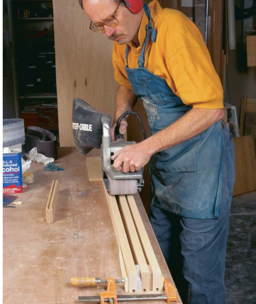
Gang narrow pieces together. This technique solves the problem of balancing a heavy machine over a single piece of narrow stock.
