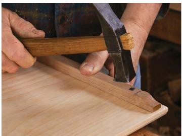
**Nail cleats to the top.** Because Follansbee uses a wide single board for the lid, he uses cleats to help keep it flat. These have decorative ogees at the front. Drive overlong nails through the cleat and the top.
