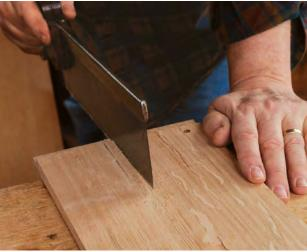
Chisel work. Strike straight down to incise the dado. Then, with a wide chisel used bevel down, bring the dado to near depth (right). Switching to a narrow chisel, split out the waste from the groove (far right), and smooth the bottom of the groove and the dado.
