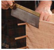
**Square pins, round holes.** Pin the back first. Use straight, square pins slightly larger than your pilot holes. The ideal pin compresses the hole a bit and fills it completely. Trim and pare the pins flush afterward.
