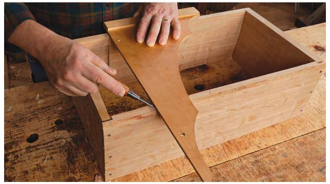
Mark till lid's length and pintles. Having the box clamped up to do this lets you mark off the actual piece instead of relying on a drawing.
