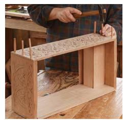
Add the till parts and front. Drop the till parts dry into the back, with the till lid open. Apply glue to the box ends and put the front in place. Patiently fiddle the till parts into position in the front, then drive the pins.
