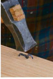
**Install the hinge in the lid.** It's easiest to press the lid onto the hinge from above. A piece of scrap protects the lid from the hammer blows. When that's done, clinch the hinges in place.
