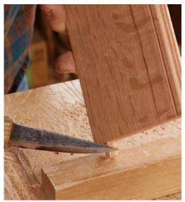
Cut the lid and pintles to shape. Start by ripping and crosscutting the lid to form the rough pintles. Then, with a knife, shave the pintles until they fit into their respective holes.
