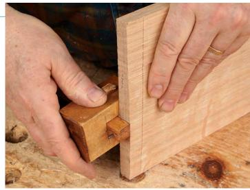
Marking gauge lays out rabbets' depth. Reference off the same surface for each joint. Follansbee uses the outside faces.
