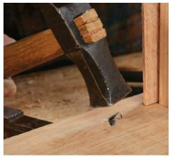
**Drive and clinch the hinges into the back.** After boring a pilot hole and hammering the hinges in place, fold over their tips with a pair of pliers. Then drive these points, like staples, into the back's inside face to secure the hinges.
