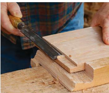
**Pare to the layout line.** Follansbee uses a long paring chisel to flatten the rabbet while bringing it to final depth.
