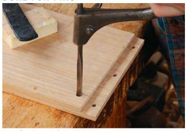
**Holes for pins and pintles.** The rabbets get pinned, so bore those holes in the box front and back now. Also bore the clearance hole for the pintles on the till's lid. This hole should not sit too close to the box's upper edge or the rabbet.
