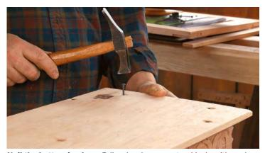
**Nail the bottom in place.** Follansbee hammers two blacksmith-made nails into the front and back and two into each end. Before driving the nails, bore pilot holes and create countersinks for the nail heads.
