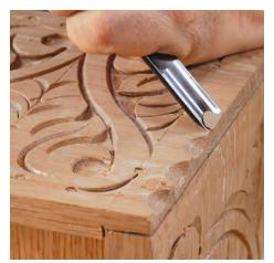
**Carve the thumbnails.** Use a deeply curved gouge and a mallet to chop thumbnail cuts into each end of the box front. Then use the same gouge to punch an echo cut right behind each thumbnail. Eyeball the spacing.
