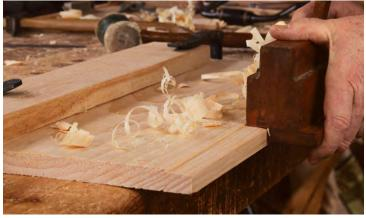
**Profile starts with a rabbet, ends with a roundover.** The lid's quarterround has a fillet above it, so the first step is to cut a rabbet. To finish the shape, Follansbee uses a smoothing plane to round over the top corner.
