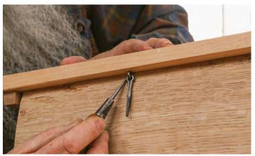
**Mark the hinge location.** Pressing down firmly on the lid, Follansbee scribes the back overhang of the lid and the eye of the hinge installed into the back. This guides him when boring the hinge's pilot hole in the lid.
