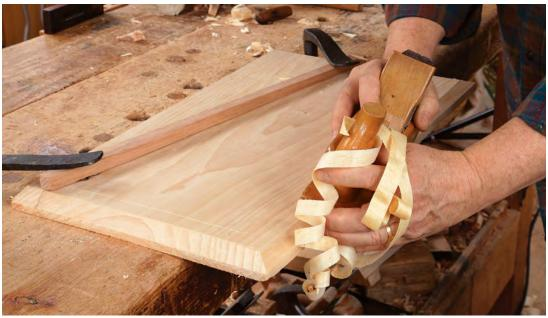
**Bottom gets a bevel.** After tracing the perimeter of the box onto the bottom, bevel the bottom's overhanging front and ends. Don't plane beyond the layout lines, or you'll create a gap under the box carcase.
