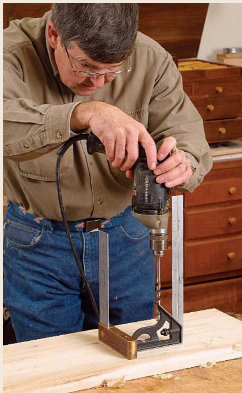
You don't need a drill press to make straight holes. Sight the bit against two squares to ensure that the hole is drilled perpendicular to the workpiece (left). Or you can use an accessory, like this drill guide from General (above), which turns the handheld drill into a mini drill press.
