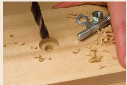
Lag bolts require stepped holes. When using brad-point bits, drill the larger hole before the smaller one.
