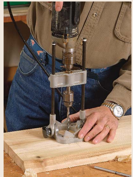
You don't need a drill press to make straight holes. Sight the bit against two squares to ensure that the hole is drilled perpendicular to the workpiece (left). Or you can use an accessory, like this drill guide from General (above), which turns the handheld drill into a mini drill press.
