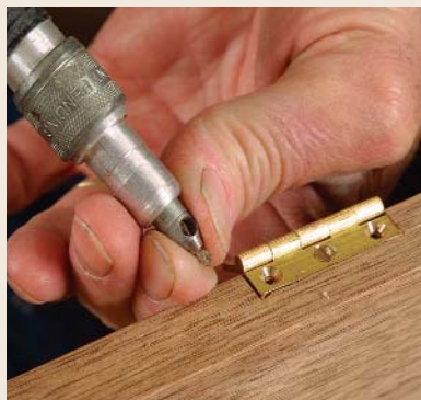
Self-centering bits help when installing hardware. Drilling for hinge screws requires precision. Self-centering bits have a tapered end on the metal housing, which centers the bit in the hinge's machined hole.
