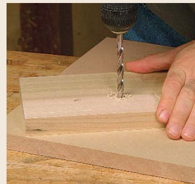
Position a sacrificial board underneath the workpiece. When wood fibers are supported, they don't tear as the bit exits the workpiece.
