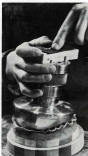
Very fragile and brittle, pearl must be sawn with a studied technique and special care. Left, with jeweler's saw and bird's mouth (the V-notched board clamped to his bench), Newman cuts a mythical sea beast from a mother-of-pearl chip. Top right, Dremel equipped with a tiny end mill routs the recess for the pearl inlay. It must fit easily, but with no gaps. Center, Newman uses an engraver's block to hold the stock when incising detail into the pearl. Engraver's blocks are necessary for good results, since engraving requires moving the work into the tool rather than the other way around, as is the case with carving wood. Engraved gouges filled with epoxy/aniline dye mixture delineate details and add depth to the finished dolphin (about twice actual size), right. Newman used black dye, but other colors would work as well.
