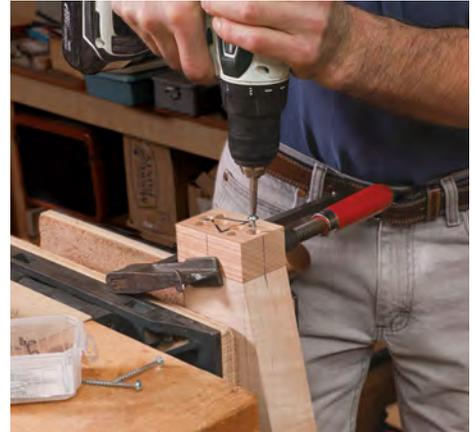
**The jig is fixed.** With the drilling jig clamped in place, Coleman drives a pair of self-drilling pocket screws to lock it to the leg.
