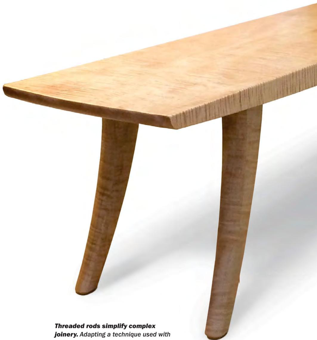
**Threaded rods simplify complex joinery.** Adapting a technique used with wooden dowels, Coleman uses a dirt-simple shopmade drilling jig and a hand drill to cut perfectly mating holes in parts that meet at odd angles. The combination of steel threaded rod and epoxy can create very strong joints in unlikely places.
