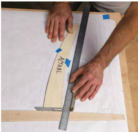
**Start with the leg.** Before making the drilling jig, cut the leg blanks' end angles. To help with layout Coleman worked from his full-size drawing to make thin plywood templates of the leg and the edge of the seat. He used a straightedge and bevel gauge to measure the angles at the top and bottom of the leg, then used those bevel gauge settings to set the miter angle on his chop saw.
