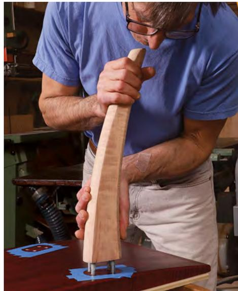
**The clincher.** Use hand pressure to push the joint together. If necessary, use clamps to bring the leg all the way home, then remove the mask of tape. While the epoxy cures, Coleman holds the leg tight with F-clamps pulling down on a pair of battens clamped to the leg. Sandpaper adhered to the inside face of the battens keeps them from shifting.
