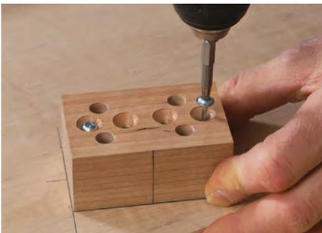
**Screw down the jig, and drill.** Aligning the drilling jig with the reference marks, screw it in place and then drill the holes for the threaded rod. Before drilling, triple check that the depth stop is properly set.
