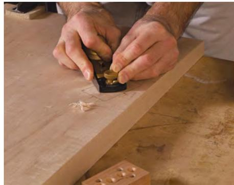
**Create a mating flat.** The underside of the seat is slightly curved, so Coleman uses a plane to create flats where the legs will be. He's careful not to erase his reference marks.
