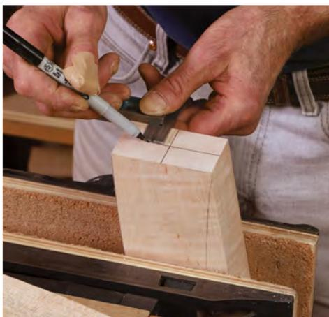
**Centerlines orient the jig.** Draw crossing centerlines on the top of the leg and extend them a little way down the sides. Then, having made a hardwood block sized exactly to the leg's width and thickness, set it on the top of the leg and transfer the centerlines to the block.
