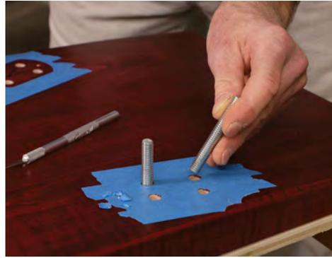
**The joints need masking.** After drilling holes for the rod, mask off the joint and a generous margin around it. Then insert the rods, dry-fit the leg, and carefully knife around the leg. Then remove the leg, the posts, and the tape inside the scribe lines.
