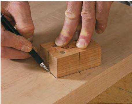
**Locate the drilling jig.** Use the centerlines to orient the drilling jig on the underside of the seat.
