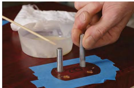
**Apply the epoxy.** Coleman uses a bamboo skewer to spread epoxy in the holes, then pushes the posts in and out to spread the glue. He also butters the top end of the leg.
