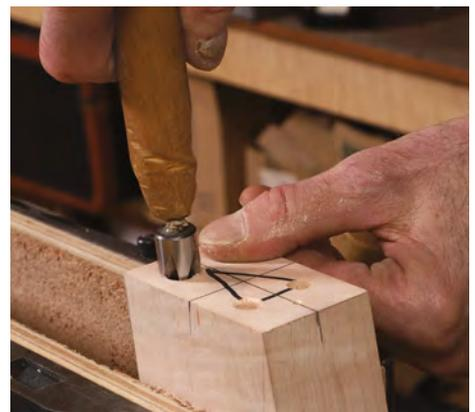
**Quick chamfer.** Countersink the rod holes to clean the rim and provide space for some epoxy squeeze-out.
