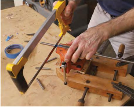
**Cut and file the rod.** Hacksaw the threaded rod to length, then chamfer both ends with a file to remove burrs and make insertion easier.
