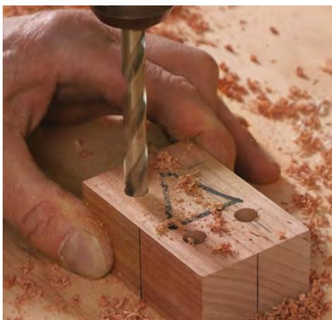
**Drill two types of holes.** At the drill press Coleman first drills the four guide holes. Then he drills four clearance holes down the middle for screws to attach the jig to the workpiece. He countersinks the clearance holes on both faces of the jig.
