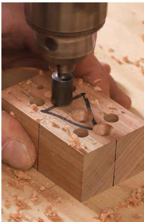
The solution came in the form of  $\frac{3}{8}$ -in. threaded steel rod instead of wood dowels, and slow-set epoxy for the adhesive. The epoxy gets in and around the threads and creates an incredibly strong and durable bond. And unlike wood dowels, the steel rods can withstand the most severe forces. This was a joint that I felt confident would hold up over time.
