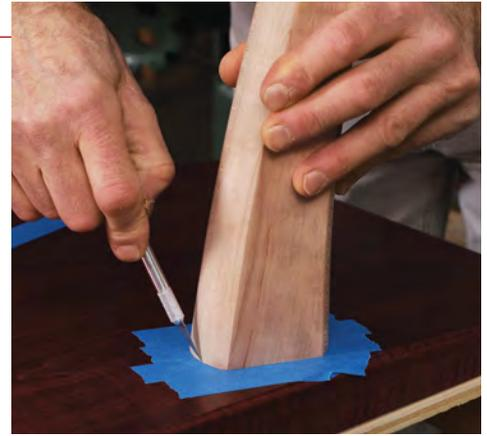
$\frac{1}{8}$  in. from the combined total depth to ensure that the rods don't bottom out and allow room for a little epoxy at the bottom.
