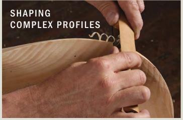
**First address the perimeter.** To shave a complex collection of curves like this chair seat, Galbert bandsaws close to the line, fairs those cuts with the shave, then creates a thin flat around the perimeter.
