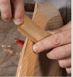
**Bring the top** and then bottom curves together at the perimeter pencil line. The top of the seat, the more noticeable surface, gets shaved first. From there, shape the bottom until there's an evenly thin line of pencil left—evidence of a perfectly crisp, multifaceted shape.
