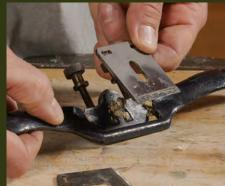
Upgrade to a thicker blade. Compared with thin vintage blades, thicker blades dampen vibration, close up the throat of the tool, and make sharpening freehand easier because of the wider bevel.
