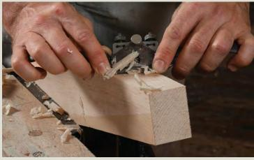
Alternate the leading hand for smoother surfaces. This crosshatching approach gives you a better feel for the surface you're shaving. Also, when you switch skewing directions, the spokeshave hits the high spots left by the previous pass, creating a more even surface.
