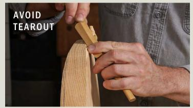
**Skew toward the longer fibers.** This keeps the fibers supported throughout the cut, limiting tearout. On a simple bevel, cutting toward the long point of the bevel is best (above). You should skew the tool so it slices up and away from the fibers (right). Otherwise, you can significantly tear out the wood.
