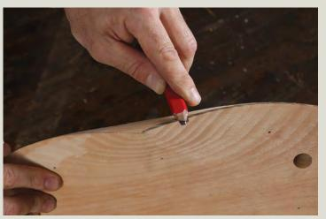
**Rub lead onto the flat.** After penciling in the flat, Galbert will shave the curves on the top and bottom of the chair seat. The penciled flat will allow him to monitor his work on the two opposing planes.
