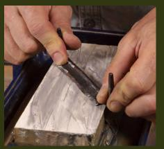
Sharpen the back on the stone's face. Apply even pressure across the blade, and angle it so the entire back remains in contact with the stone.
