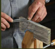
Sharpen the bevel on the stone's edge. Use this approach when the tangs are too close together to use the stone's face or the blade isn't perfectly straight across.
