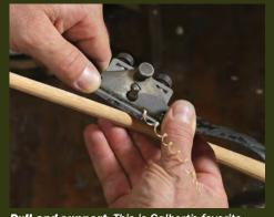
**Pull and support.** This is Galbert's favorite grip. It's the same as the basic pull, except he braces the stock underneath with his fingertips, stabilizing the workpiece and giving tactile feedback on the cut.
