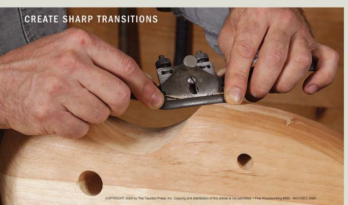
Start off the surface for sharp transitions. When two distinct shapes meet at a sharp edge, angle the shave so that only a small portion of the sole is firmly bedded at the start. This lets you smoothly slice into the cut instead of abruptly contacting the blade, which can cause chatter and an uneven cut.
