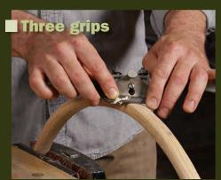
**Push.** When pushing the tool, Galbert's thumbs comfortably fit into the areas behind the body of the tool and drive the motion. He uses a delicate grip, and focuses pressure right above the sole with his index fingers.
