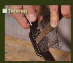
File the blade bed flat if necessary. With vintage spokeshaves, check that the bed is flat. If it's not, the blade will be poorly supported during the cut. File the bed if it's off, checking your progress frequently.
