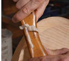
**Adjust the cut by rotating the tool.** You can take light or heavy cuts simply by pitching the tool slightly more forward or back. This allows you to hog off material quickly and then take light finish passes without fiddling with blade adjusters.
