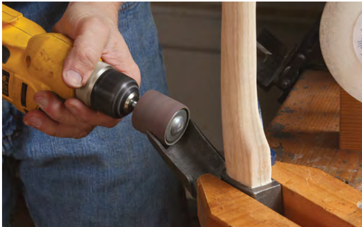
Grind the inner bevel with a sanding drum and drill. A drum with a radius slightly smaller than the adze edge helps create an even grind. The inner bevel can be quite small, but much depends on the thickness of the steel near the edge.
