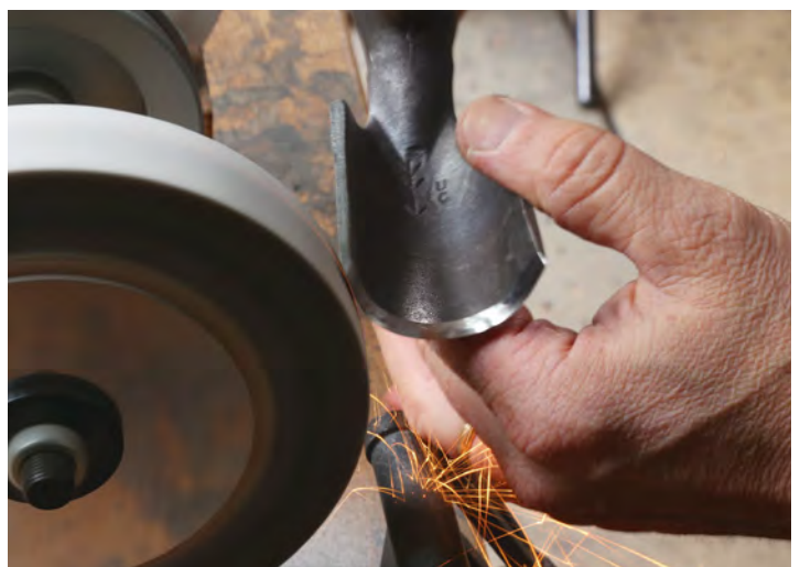
Grind the outer edge corner to corner. Fisher rests his left hand on the tool rest and supports the head with his fingers. His right hand holds near the poll. Together, they rotate the adze head, grinding the outer bevel from corner to corner. He sights from above, uses a very light touch, and takes his time while making successive passes. Grind almost to the edge.
