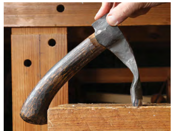
Test the hang. With the cutting edge against a flat surface, extend the handle off the edge so that the pivot point of the swing hangs free. The cutting edge should be about 90° to the surface.
