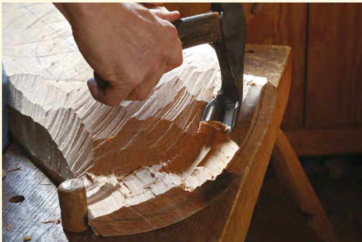
Super for sculpting. An adze, essentially a carving gouge that you swing, can quickly hog away green wood to form pleasing curves, like on the underside of a bowl handle or the crook of a spoon.
