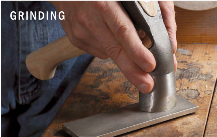
Joint the edge on a coarse stone. This lets you start with an even surface. A small flat across the whole edge tells you when you're done.
