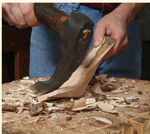
Super for sculpting. An adze, essentially a carving gouge that you swing, can quickly hog away green wood to form pleasing curves, like on the underside of a bowl handle or the crook of a spoon.
