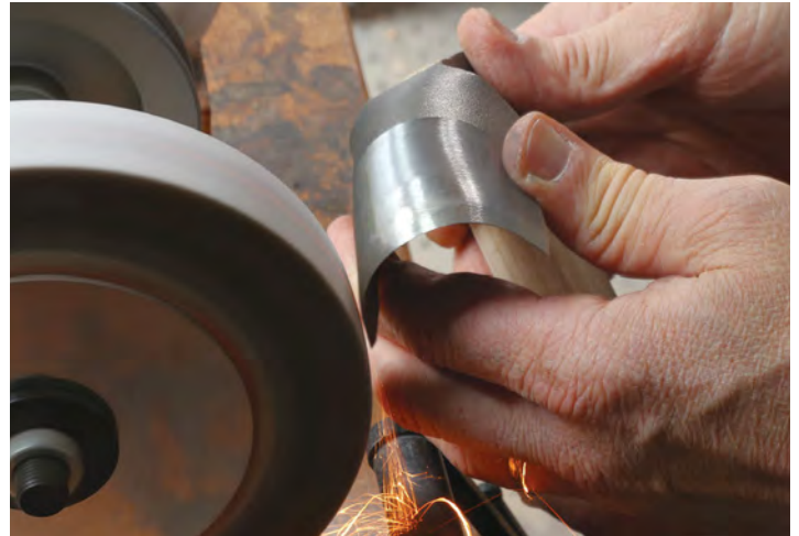
Joint the edge on a coarse stone. This lets you start with an even surface. A small flat across the whole edge tells you when you're done.
