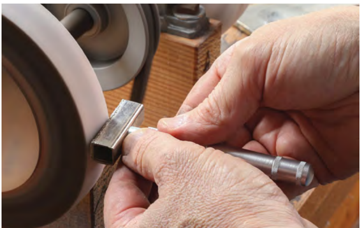
Dress the wheel with a slight crown. Use a diamond wheel dresser, leaving a slight hump in the middle of the wheel. This crown allows for greater control and just a bit of hollow grind.
