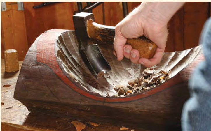
A boon for bowls. There's a lot of material to remove when hollowing a bowl. A well-tuned adze with the right geometry handles this task surprisingly fast.
