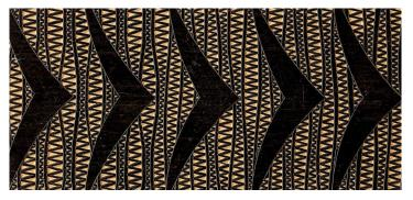
Dyed veneer on solid wood. Cutting through the veneer reveals the contrasting color beneath. As with the previous methods, before carving bring the top layer to a finished surface with five to six coats of oil/varnish, then carve. Finish up with two to three coats of a thinned-down mixture.
