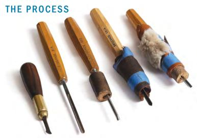
A handful of tools. Madsen's basic carving kit is a minimal five tools. She uses Swiss-Made tools to cut the marks: two gouges, 8/3 and 8/4; two V-parting tools, 12/4 and 13/4; and a knife.
