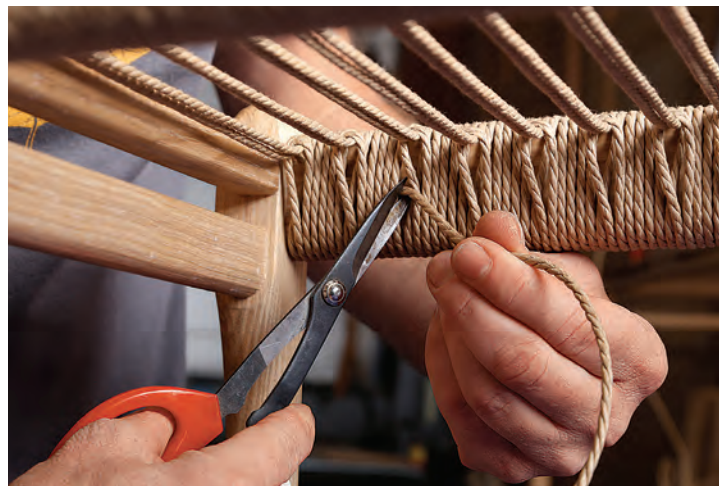
5. Continue in this manner until about 2 in. from the end of the back rail. Finish with the dowel technique.
