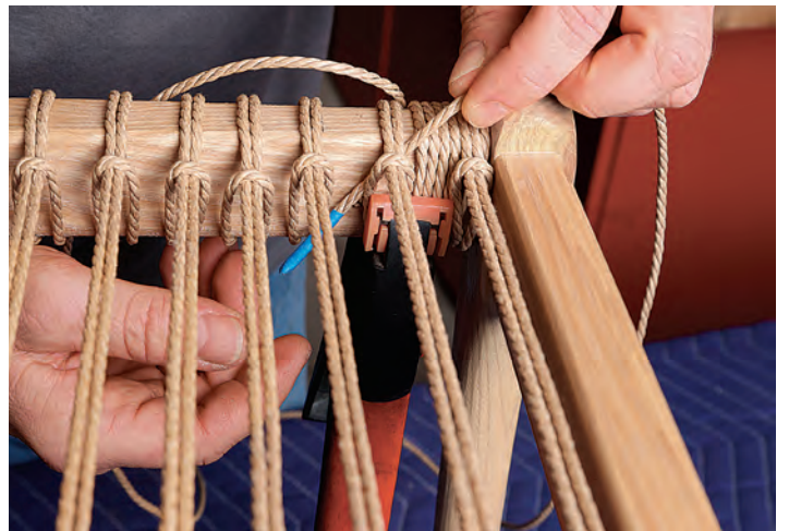
4. When the area is filled, move to the area between the second and third warp pair by passing the cord under the loop of the second warp pair.
