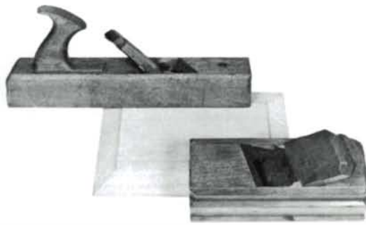
Planes in use. Top, the A. Smith plane from previous photo; bottom, English panel plane, 3 in. wide by 8 in. long, has adjustable fences on sole and side for width and depth control.
