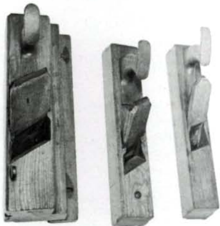
Three panel-raising planes, circa 1800. Left, raising jack made by J. Butler of Philadelphia, has adjustable fence and depth stops, and nicker cutter ahead of skewed iron. This prevents tear-out when working across the grain. Plane at center was made by A. Smith of Rehoboth, Mass.; right was made by S. Kimball. All three planes are 14 in. long, and range from 2 1/4 in. wide to 3 1/4 in. wide.
