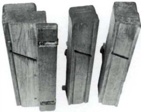
Three panel-raising planes, circa 1800. Left, raising jack made by J. Butler of Philadelphia, has adjustable fence and depth stops, and nicker cutter ahead of skewed iron. This prevents tear-out when working across the grain. Plane at center was made by A. Smith of Rehoboth, Mass.; right was made by S. Kimball. All three planes are 14 in. long, and range from 2 1/4 in. wide to 3 1/4 in. wide.
