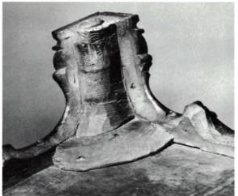
G: Typical bracket-foot construction, as in this view of the Massachusetts slant-top desk, (also shown in photo D) employs a corner glue block with the grain running perpendicular to the grain of the bracket members. Cracked bracket feet are common. Note that the base-molding glue blocks run all the way into the corner, unlike the glue-block construction shown in photo F.
