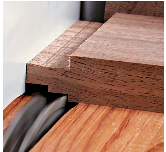
Dado set is the secret. Assemble the outer blades and inside chipper blades to make a wide cut. With this setup, you can cut a tenon in one or two passes.
