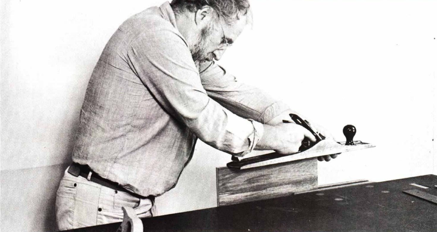
Finish the edges of the veneered panel with a jointer plane, after first trimming with a veneer trimmer, router or knife.
