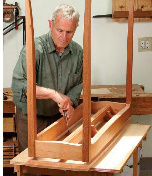
**Use a wooden drill stop.** This regulates the depth of the screw hole in the tabletop. This is not the time to use a piece of tape as a depth guide and risk it slipping. That would give you a pilot hole straight through the top.
