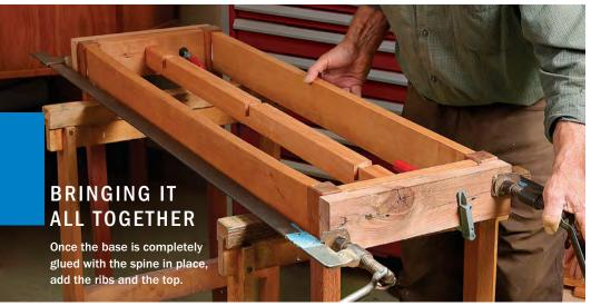
**The final glue-up.** Once the first phase (short aprons to the legs) of the assembly is dry, glue the long aprons and spine between them.
