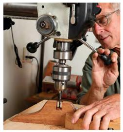
Connect the rib to the spine. Drill for the screw that will attach the rib to the spine. Drill the smaller diameter pilot hole first. After transferring that hole's location to the spine, drill a larger clearance hole in the rib, and finally a countersink for the screw head.
