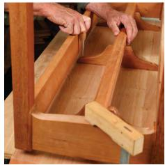
Marking for the screw holes into the top. Hold the awl perpendicular to the top, ideally centered in the slotted holes.
