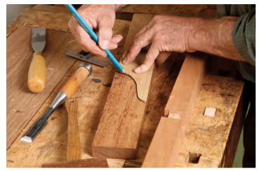
Lay out the shape. For the sake of symmetry, the template has only one side. Flip the template over to mark the opposite end of the rib.
