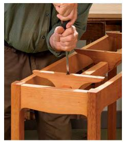
**Attach the ribs to the spine.** Welter uses #12 screws to fasten the parts together. The halved joint is very snug; no glue is necessary.
