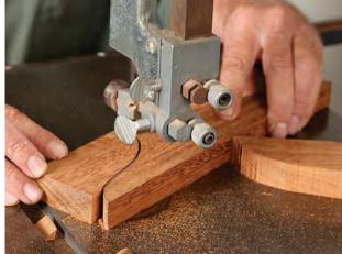
Notch and shape the rib. With the rib still square, cut the notch with repeat crosscuts on the tablesaw using a miter gauge. Once the notch is cut you can cut the rib's shape on the bandsaw.
