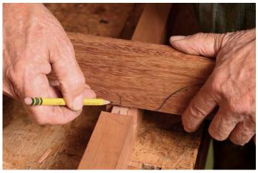
Lay out the notch. Line up center marks on the rib and the spine. Then lay out the notch in the rib.
