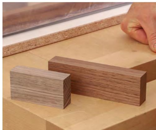
**Is it done yet?** Having placed samples in the chamber with the furniture, Gochnour pulls one out to check the progress and compare it with an unfumed sample.
