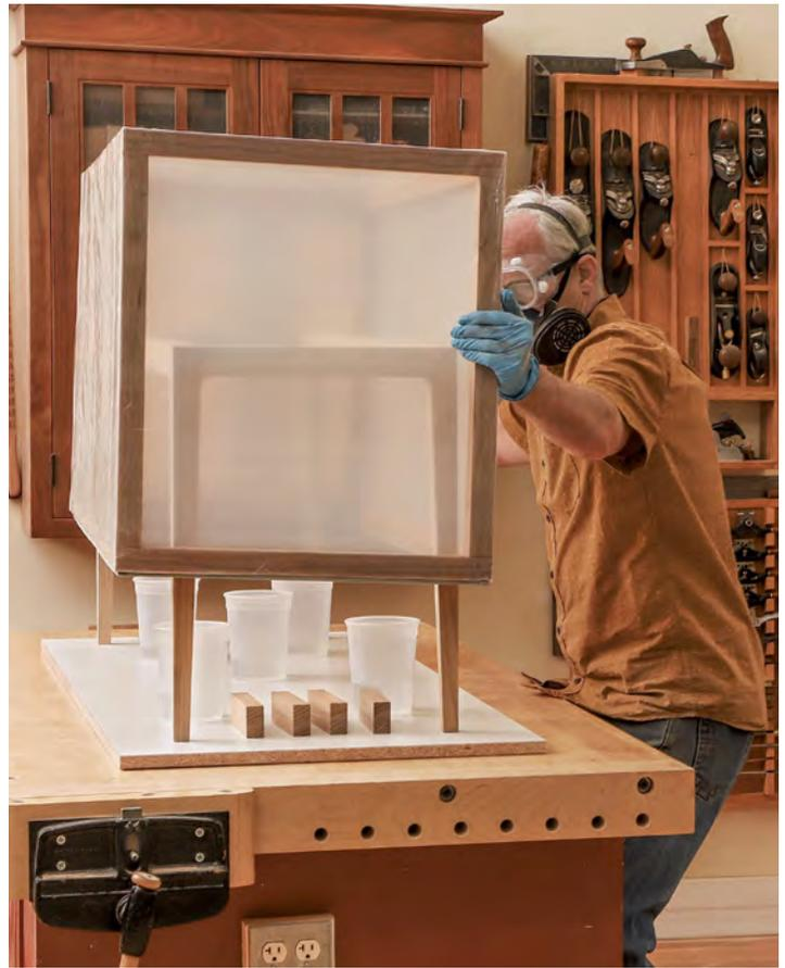
**Lower the tent.** After the chamber is in place on the melamine base, Gochnour puts a piece of MDF or other heavy sheet material on top of the chamber to weight it down and ensure a good seal at the bottom.
