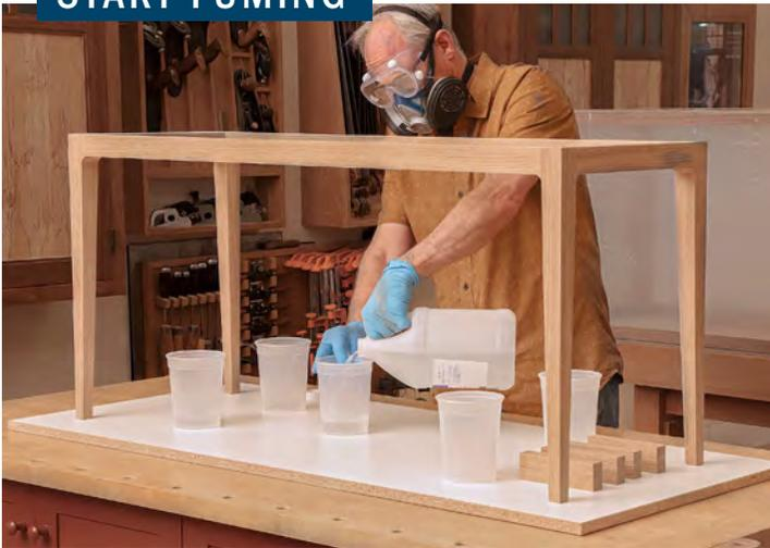
**Pour the potion.** To reduce the chance of splashing and spilling, use deep containers and fill them to about 1 in. deep with aqueous ammonia. Work in a well-ventilated area and wear gloves, goggles, and a respirator.
