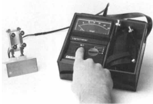
Part of a dry-kiln control system, this cellulose wafer (left) reacts almost instantly to changing RH levels to yield EMC readings directly, without reference to conversion charts. Available from Lignomat USA (14345 NE Morris Court, Portland, Ore. 97230), the device currently costs $80 without the meter, mostly due to the cost of the kiln-proof holder—the wafers themselves, which are replaced every three weeks, are only about 35¢.
