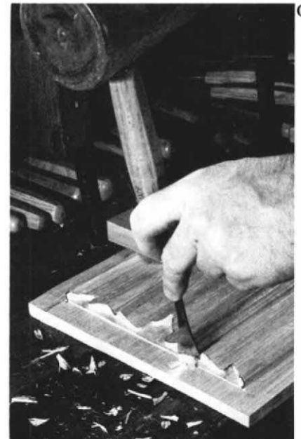
Set in by driving vertical cuts to within \frac{1}{16} in. of the background.
