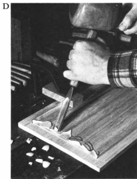
Bevel between the lines with a gouge, leaving bottom edge of 'cloth.'
