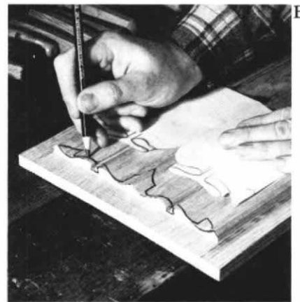
Make a template of the end folds and trace it on the work.
