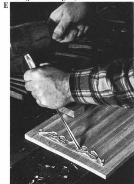
Outline the edges with a V-tool, cutting with the grain as much as possible.
