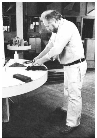
The main difference between sharpening a chisel and a plane iron is the pressure applied to the tool. The handposition, as shown in the two photos at right, is basically the same, Rear down hard on the wide iron, varying the pres-sure from left to right every few strokes, to round the edge slightly. Maintain constant, light pressure on a narrow tool. Here, Kirby uses a Japanese waterstone, kept wet by squirts from a plant sprayer.
