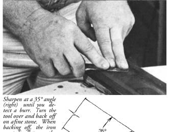
tool over and back off on afine stone. When backing off, the iron must lie flat on the stone (as shown at left and above). Use the fingers of both hands
