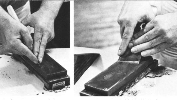
lubricant is to keep the edge of the tool cool, to smooth the sharpening action, and to float away metal and stone debris, thereby helping to prevent plugging or glazing of the stone's abrasive surface. If you have oilstones, the type of oil is also a matter of preference. A light machine oil such as 3-in-1 is good. Motor oil cut with kerosene is popular, and straight kerosene is suitable on a fine stone.
