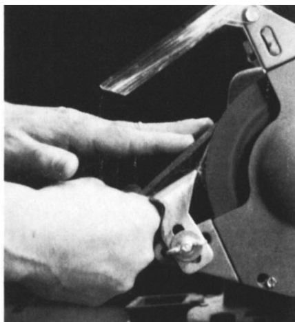
The proper position for the index finger of the right hand, which rides against the bottom of the tool rest, will produce an initial grind mark about in the middle of the bevel, left. If the grind mark is too high, lower your finger; if the mark is too low, raise your finger. While grinding, second photo from left, the blade does not necessarily rest on the
