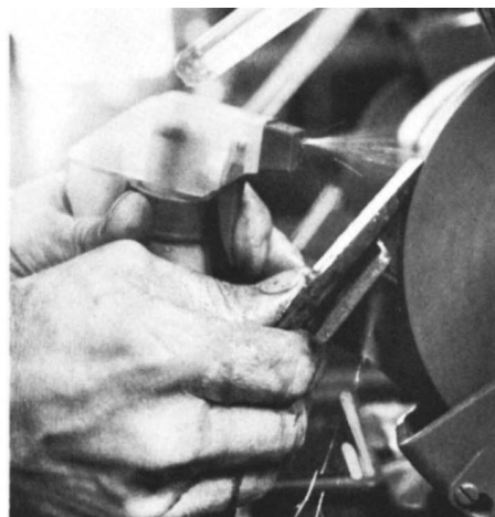
flat of the tool rest; the position of the index finger determines the bevel angle. As the grind nears the edge of the blade, it becomes easy to overheat it. Learn to control the tool with only your right hand, freeing your left to spray the edge with water as you grind, second photo from right. At right, the hollow-ground bevel directly off the grinder.
