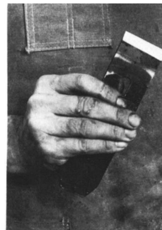
flat of the tool rest; the position of the index finger determines the bevel angle. As the grind nears the edge of the blade, it becomes easy to overheat it. Learn to control the tool with only your right hand, freeing your left to spray the edge with water as you grind, second photo from right. At right, the hollow-ground bevel directly off the grinder.
