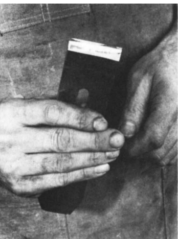
The proper position for the index finger of the right hand, which rides against the bottom of the tool rest, will produce an initial grind mark about in the middle of the bevel, left. If the grind mark is too high, lower your finger; if the mark is too low, raise your finger. While grinding, second photo from left, the blade does not necessarily rest on the
