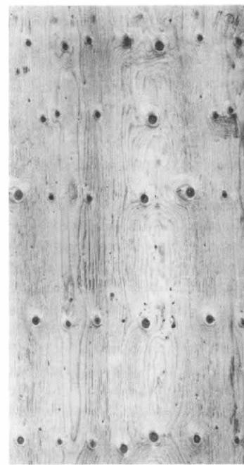
Coniferous trees, left, are characterized by excurrent form, i.e., a dominant stem from which whorls of lateral branching occur at regular intervals, or nodes. The pattern is often present on plywood made from rotary-cut softwood veneer, right.
