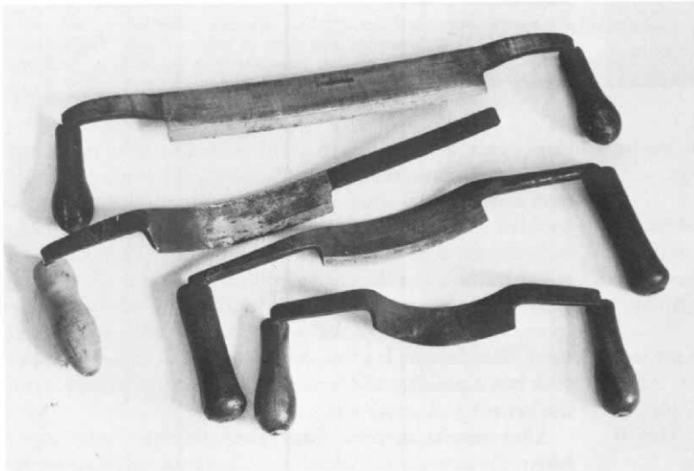
Various drawknives satisfy different needs. Above, from top to bottom, straight blade is for general-purpose work. The second can be used to slice wood with the blade at an angle or, with its straight handle out, to chamfer the inside of a bucket rim. The third has a slightly curved blade with the bevel on the concave face—best for light cuts and finishing work on flat surfaces. At top right, a similar drawknife, but with round, French-style handles, takes a fine shaving. The fourth drawknife has a radically curved blade with the bevel on the convex face. This tool makes fast work of hollowing out barrel staves, removing large shavings (photo, right). Also known as an inshave, it is the drawknife equivalent of the scrub plane.
