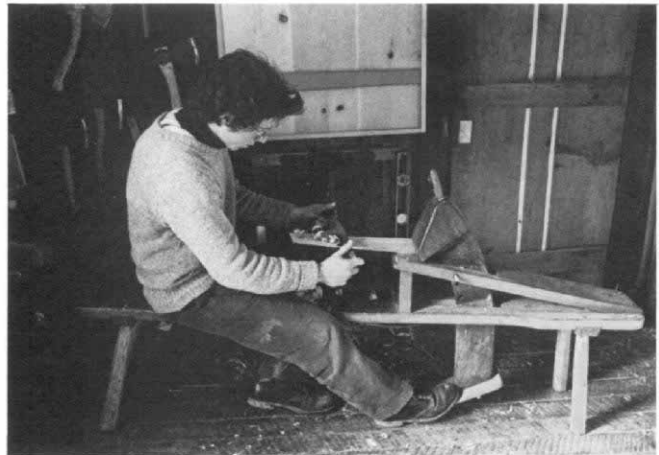
Drawknife and shaving horse offer an ideal combination of direct shaping and quick, sure gripping of green stock.
