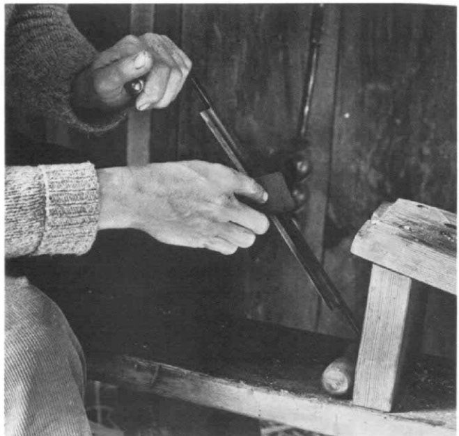
Drawknife and shaving horse offer an ideal combination of direct shaping and quick, sure gripping of green stock.
