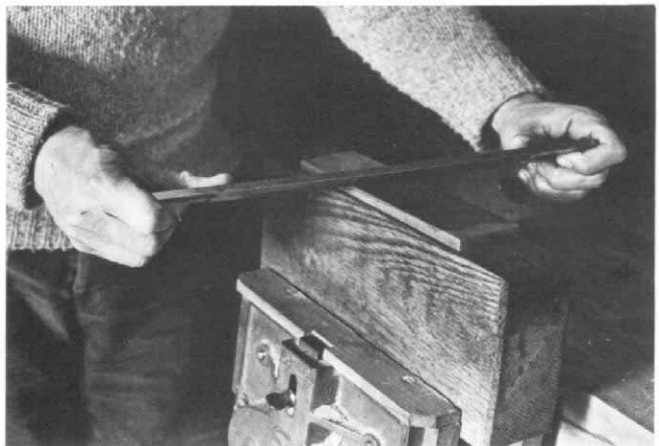
Two methods of sharpening drawknives. A Swiss cooper teaches supporting the drawknife on the shaving horse, center, and rubbing a handstone first over the bevel, then over the flat face, moving it up and down the length in small circles. A Swedish woodworking instructor teaches mounting the stone in a block of wood held in a vise, above. The drawknife is drawn diagonally over the stone, toward you and toward your right, so the entire length of the blade is whetted in each stroke.
