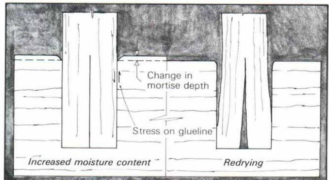
Fig. 8: In moisture extremes, typically high moisture content followed by redrying, the changing depth of the mortise and compression set near its mouth shear the glue line. The split tenon accommodates stress at the bottom of the hole, but racking will soon break it loose.
