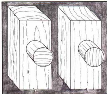
Fig. 6: The optimum condition (left): tangential movement coincides in both mortise and tenon, while the lesser radial dimensional change in the tenon opposes the stable long grain of the mortise. At right, tangential movement varies the depth of the mortise and may "walk" the tenon out, while compression will cause the greater change in tenon height.
