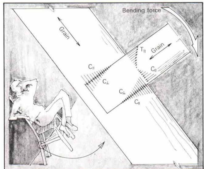
Fig. 1: Tilting back in a chair racks the joints. The rung tends to bend, causing axial stresses (tension,  $T_{||}$  and compression,  $C_{||}$ ). In turn the rung tenon bears against the mortise walls, compressing the rung perpendicular to the grain ( $C_{\perp}$ ) and the mortise parallel to the grain ( $C_{||}$ ).
