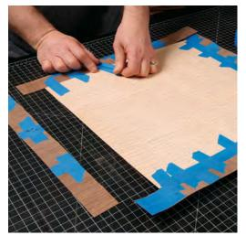
Start by taping the border of face bandings to the central field of veneer. Make sure to center each piece of banding, and just let the ends overlap. Creating clean miter joints on these pieces to prevent chipping and blowout. Then flip over the sheet so you
