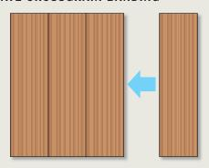
2. Crosscut the veneer panel into four crossgrain strips, each long enough to span the table and wide enough to yield a matched pair of face and edge bandings.
