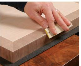
Final surface prep. Make short strokes across the edge, using a small, hard sanding block. Then apply a very fine roundover to the corners, hand sanding with folded 320-grit paper, and the joint disappears.
