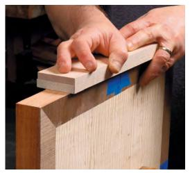
Clean up the overhang. After gluing the veneer to the substrate, use a flush-cutting bit to trim the overhang (left). Then attach 120-grit paper to a long, hard block and sand away any remaining glue or veneer (above). Note that the plywood substrate was pre-edged with mahogany veneer to keep the layers from telegraphing through the show veneer.
