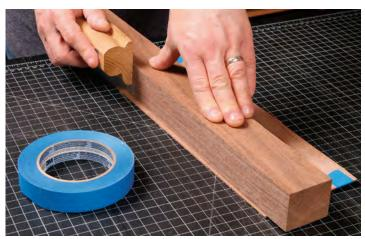
**Trim the stack.** Figure out how much crossgrain veneer you need, tape it into a stack, and trim the edges parallel to the grain. Use light pressure and multiple passes to cut cleanly through the four plies.
