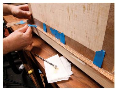
**One strip at a time.** After applying glue, align the edge strip carefully and tape it in position. Its extra width makes it easy to align the grain perfectly. A thick cork-lined caul distributes the clamping pressure evenly, and a second caul protects the opposite edge of the panel. Wait a couple hours, trim the overhang, and move on to the next strip.
