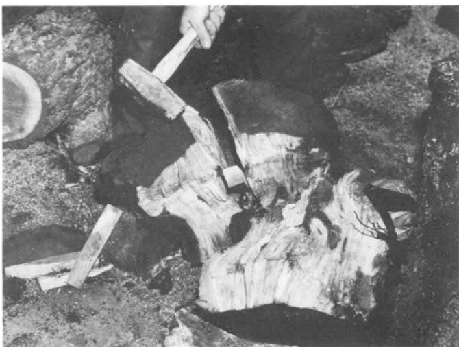
Wedges are used to split a cherry stump containing pockets of dirt and rocks. Be sure to split through the pith.
