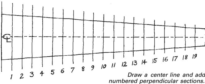
Draw a center line and add numbered perpendicular sections.
