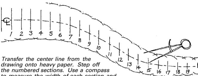
Transfer the center line from the drawing onto heavy paper. Step off the numbered sections. Use a compass to measure the width of each section and swing arcs at the corresponding marks along the curved line. Connect the crests and this is your pattern.
