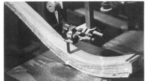
Use the form and shims to lay out the finished width on the lamination and bandsaw to size.
