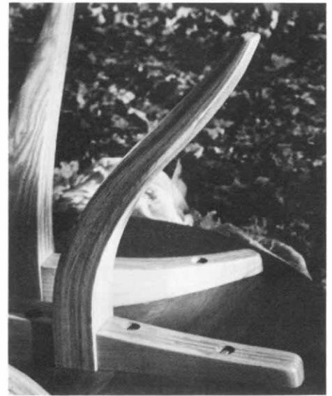
Ash legs of table are single-tapered lamination. Table top is teak, and measures 57 in. diameter. Table is 29 in. high.
