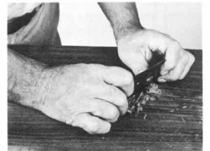
Block and clamp hold curly spot down while glue cools; strip of heavy paper along seam keeps it closed until glue dries. Then a sharp scraper cleans off paper and glue.
