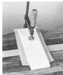
Block and clamp hold curly spot down while glue cools; strip of heavy paper along seam keeps it closed until glue dries. Then a sharp scraper cleans off paper and glue.
