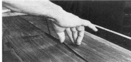
Saw through both veneers at once, carefully lift top sheet and peel away scrap beneath.
