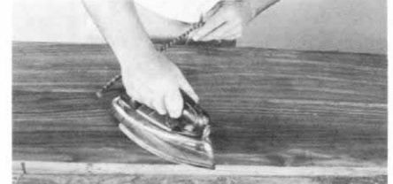
A hot iron remelts the glue in a troublesome spot. Then go over it with the hammer.
