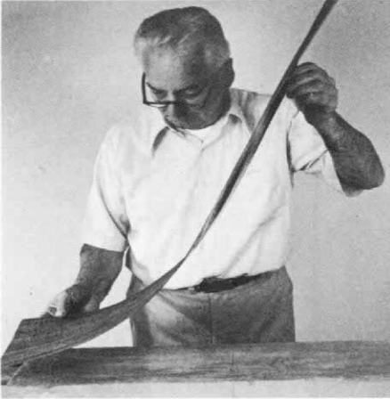
Lay veneer face down in glue. The glue that smears on it will help hammer slide easily.
