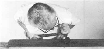
Lean your whole weight on the hammer, squeezing the glue toward the edges.
