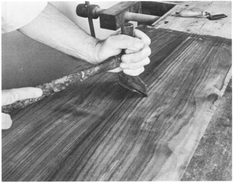
With both sheets stuck and the seam trimmed, reheat with the iron and push hard with the hammer to squeeze the excess glue out through the line of the joint.
