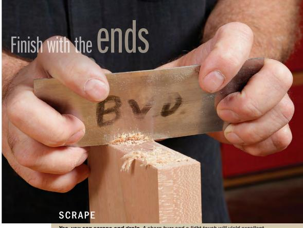
**Yes, you can scrape end grain.** A sharp burr and a light touch will yield excellent results. The chamfers you made will help prevent splintering the edges.
