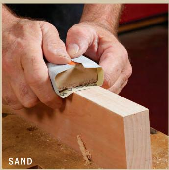
**Use your grip for control.** Van Dyke uses his fingers like outriggers, letting them slide along the faces of the board to keep the sanding block flat and on track.
