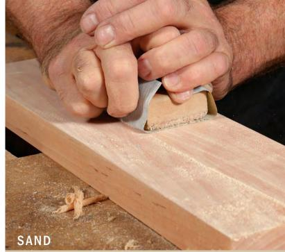
**Long strokes.** Use 320-grit sandpaper to further smooth the surface left by the scraper. Van Dyke wraps his sandpaper around a hard felt-faced or cork-faced block. He applies firm downward pressure while taking long passes with the grain of the board.
