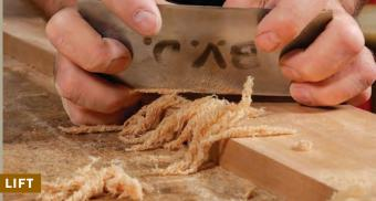
**Touchdown and liftoff.** Don't try to force the scraper into the wood and then push. Instead, approach the cut gently and smoothly. After the scraper makes contact with the board, take light strokes with a skew cut. Finish by lightly lifting off the wood.
