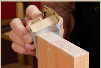
Sand for glassy end grain. After sanding across the scraped ends, sand the chamfers in two strokes. Taking more than two or three passes will muddy the clean, even chamfers left by the block plane.
