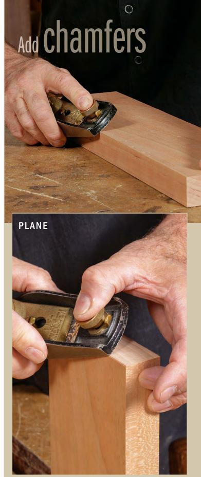
**Lightly chamfer all edges.** Skew a block plane when relieving the hard 90° edges. Take long, even passes for sharp, uniform chamfers.
