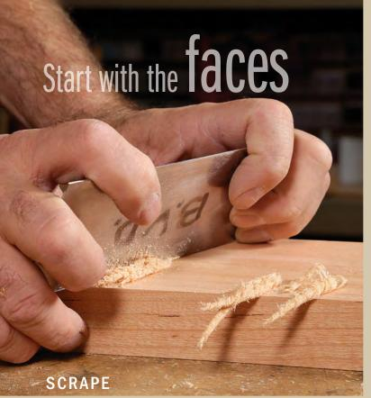
**Proper form.** Hold the tool as vertical as possible while still cutting, and bow it slightly. Press your thumbs together behind the cutting edge and keep them half on the scraper and half on the board.
