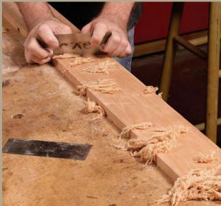
**Overlap short strokes for an even surface.** Start at the far end of the stock and, using short, overlapping strokes, move backward while scraping into the section that you just finished.
