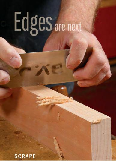
**Scrape with care.** Again, keep a part of your hand in contact with the board and use a light touch, especially when near the edges. A heavy touch here will destroy a crisp edge in a heartbeat.
