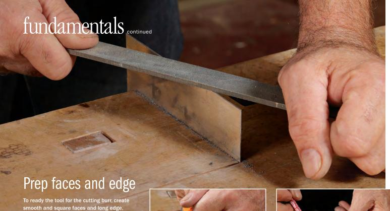
Joint an edge square with a file. The edge is ready when the file makes a consistent pass, leaving an even scratch pattern. Van Dyke uses a 10-in. mill bastard file.
