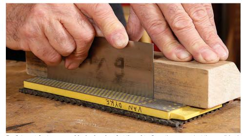
**Register against a square block when lapping the edge.** Draw the scraper (not the wood) back and forth over the stone. The wood helps you maintain 90°. Again, aim for a uniform polish across the whole edge before moving to finer stones.
