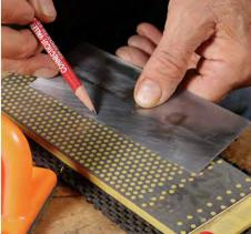
**Look for a uniform scratch pattern.** Work your way up to finer stones, lapping the face only near the jointed edge. There's no need to lap the middle of the scraper.
