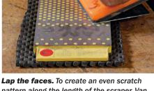
**Lap the faces.** To create an even scratch pattern along the length of the scraper, Van Dyke uses a push pad, tipping it slightly to direct pressure along the edge.
