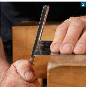
Turn the burr. Finally, angle the burnisher ever so slightly before drawing it up and across the edge two or three times. Don't exert a lot of pressure. A small sharp burr is easier to use and will last longer than a big one.
