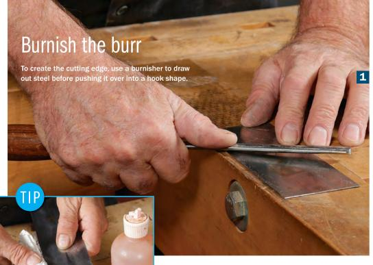
Draw out the steel. Hold the burnisher at a very slight angle to the face, skew it, and pull it along the scraper while pressing it firmly against the face. This creates a slight burr along the edge.
