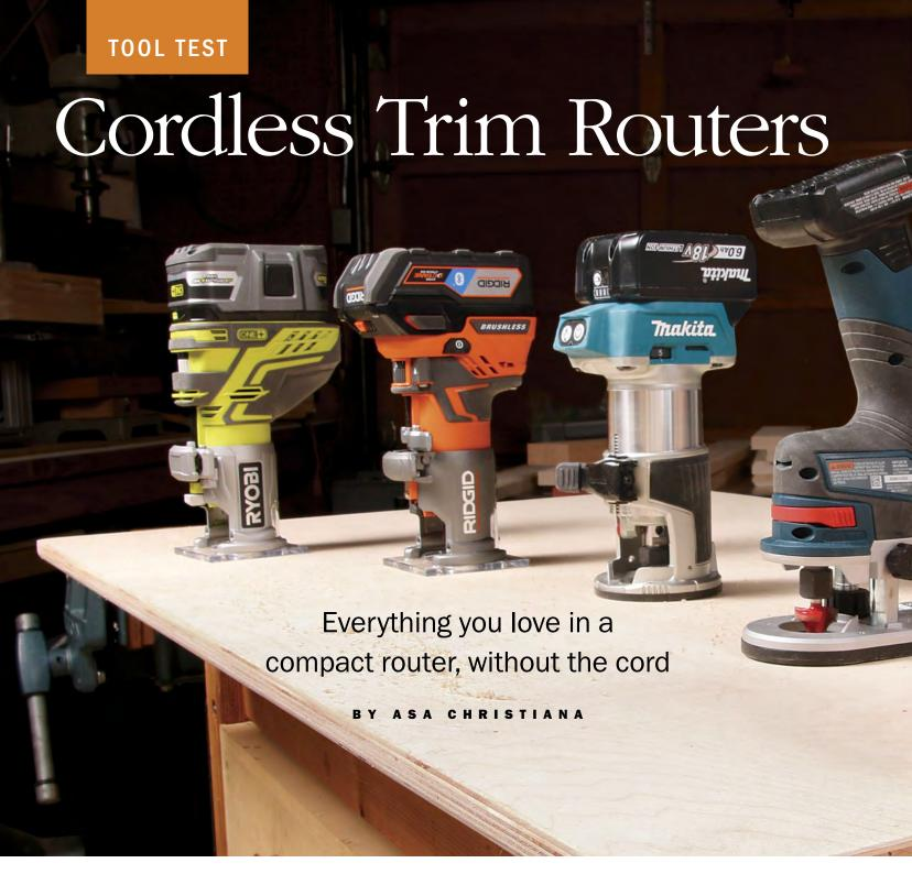
hile battery power makes any power tool more convenient, with a router cutting the cord improves safety and cut quality, too. Without the troublesome tether dragging behind and catching on corners, your pace and your path are steadier, and you can focus your hands and eyes on the work. The perks are especially apparent on a trim router, a tool built for agility and control that can still stand up to most router tasks shy of full-size mortises and big molding profiles.
