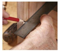
**Pencil the inside edge.** With the divider dryfitted in the case, push a straightedge against the case interior to locate the inside edge of the miter.
