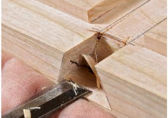
Refine the housing with a chisel. Use a paring chisel to nail the perfect fit. A router plane can help level the bottom of the joint. Just add spare cock bead stock in the rabbet to stabilize the base of the router plane.
