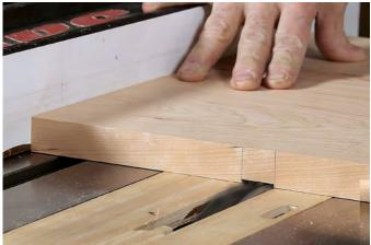
Dadoes first. Set the blade width to match the divider's thickness. When cutting the dadoes, register the end of the case side against the rip fence.
