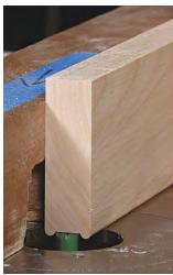
**Bead the dividers.** Using the same setting as for the loose bead stock, rout two beads into the front edge of the divider (left). To remove the waste between beads on the divider, reset the fence and use a straight bit (right).
