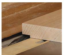
Rabbets second. Using an L-fence that extends above the blade to set the width of the rabbet (above), Neptune cuts to the same depth as the dado. The bead stock should extend beyond the front edge of the case the width of the bead radius (right).
