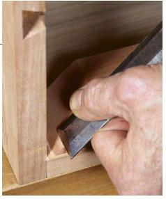
The case top and bottom get miters, too. Clamp an angled block to the case to guide the chisel. The miter should end at the inside corner of the case.
