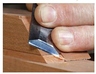
**Pare the first miter on the end.** This paring block has a rabbet that fits the stock, allowing for easy and consistent registration.
