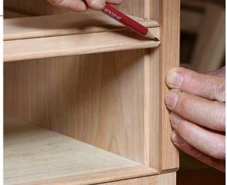
Mark and cut to length. Hold the loose cock bead so the tip of the first miter aligns with the tip of the case's miter. Pencil a line. This will be the outside edge of the loose bead's second miter. Cut the piece to length, then use the same rabbeted paring block. Work carefully for a gapfree fit (below).
