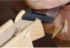
mill the loose cock bead stock. For the best grain and color match, cut wood for these pieces from the same board as the case sides, ripping off a 1-in. strip adjacent to the front of the case side, and resawing it. The resulting long strips will give you several shots at a good miter.
