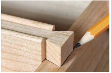
**Transfer the dovetail to the case.** With the divider in the dado, trace around the tail with a sharp pencil. Also, mark its width inside the case.
