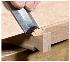
**Pare the miters.** This miter should end at the base of the dovetail. Using a 45° paring block, take light cuts. Score the front edge before mitering it to ensure a clean cut.
