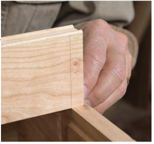
Trim the dovetail to width. Keep the dovetail between 5% in. and 1 in. wide (right). Anything more begins to weaken the case side. Neptune cuts close to his lines at the bandsaw (far right) before paring to them with a sharp chisel.
