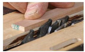
Set the blade height to match the bead. If your dado stack leaves a less-than-perfect surface, lower the blade slightly and clean up the joint with a rabbet and router plane. Just make sure to plane the rabbet and dado to the same depth.
