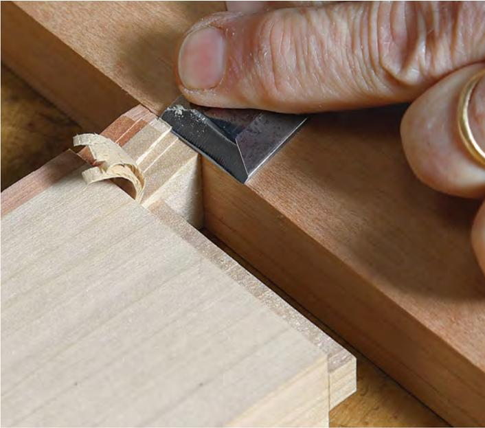
**Pare both sides of the dovetail using the angled paring block.** Begin by rough-chopping the shoulder away from the line and splitting off the waste before taking narrow shavings with a sharp chisel.
