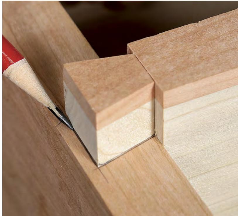
**Housing for dovetail.** Pencil around the tail, then use a saw, chisel, and router plane to form the housing.
