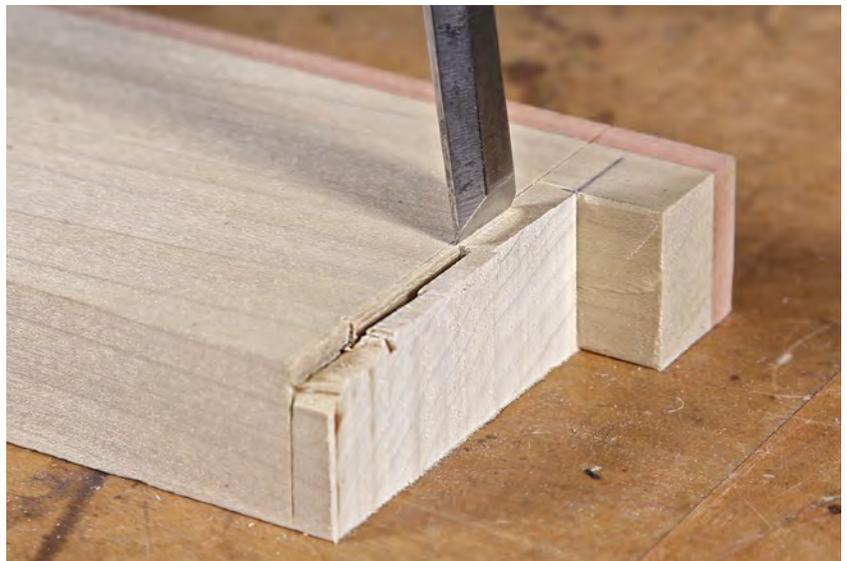
in from the end. Finish by paring the shoulder back to the scribed line and the tenon flush with the paring block. Keep the back of the chisel flat against the block. I recommend a wide chisel for more support on the block.
