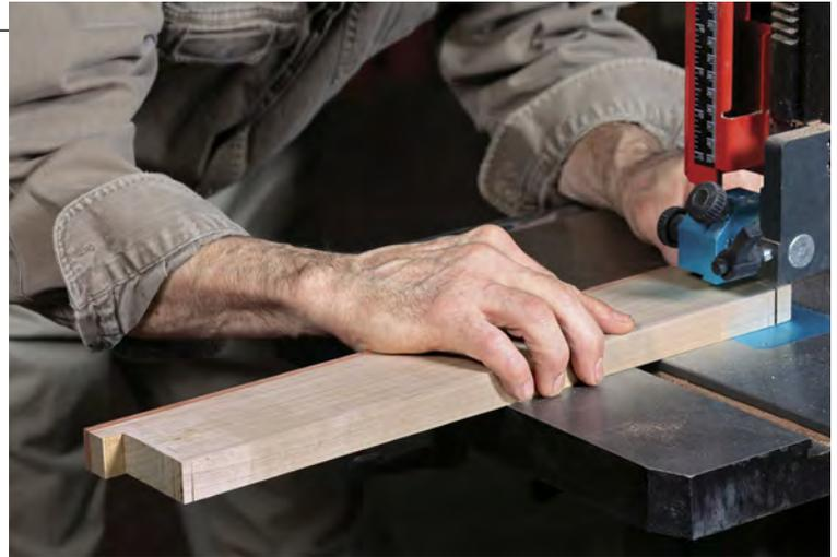
**Trim the waste.** Cut the stub tenon to length and the dovetail to width. Neptune uses a bandsaw and cleans to the line with a chisel.
