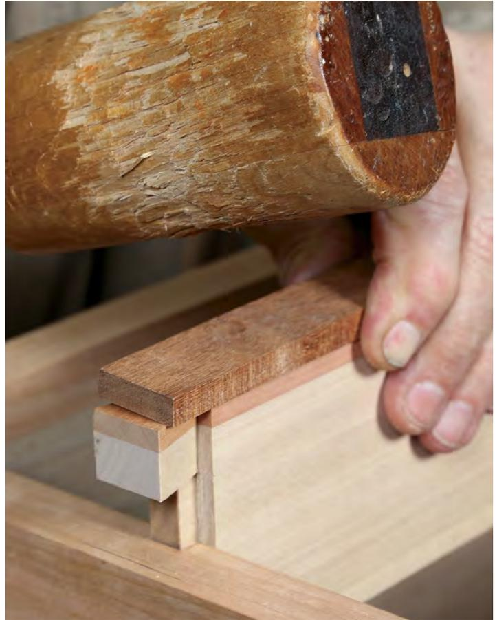
**Tap in the divider.** Use a scrap block to protect the workpiece as you drive the divider into the case.
