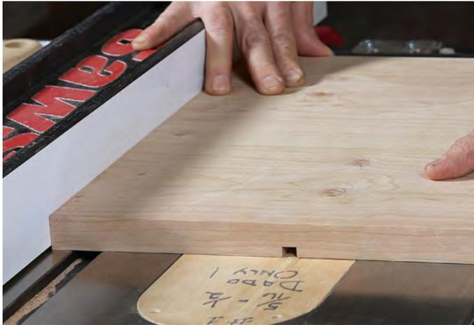
**The dado size depends on which dovetail you pick.** If you are making a stepped-dovetail divider and your dado stack's outside blades leave deeper scoring marks, level the bottom of the case dados with a router plane. Otherwise, the show face of the joint will have triangular gaps at the shoulder.
