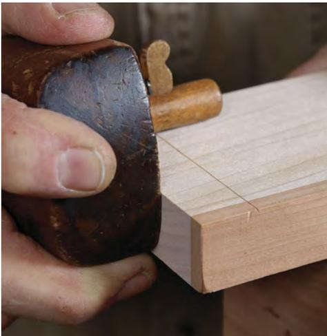
**Scribe the shoulders.** Set the divider in place and check that the dovetail shoulders align with the inside of the case (right).
