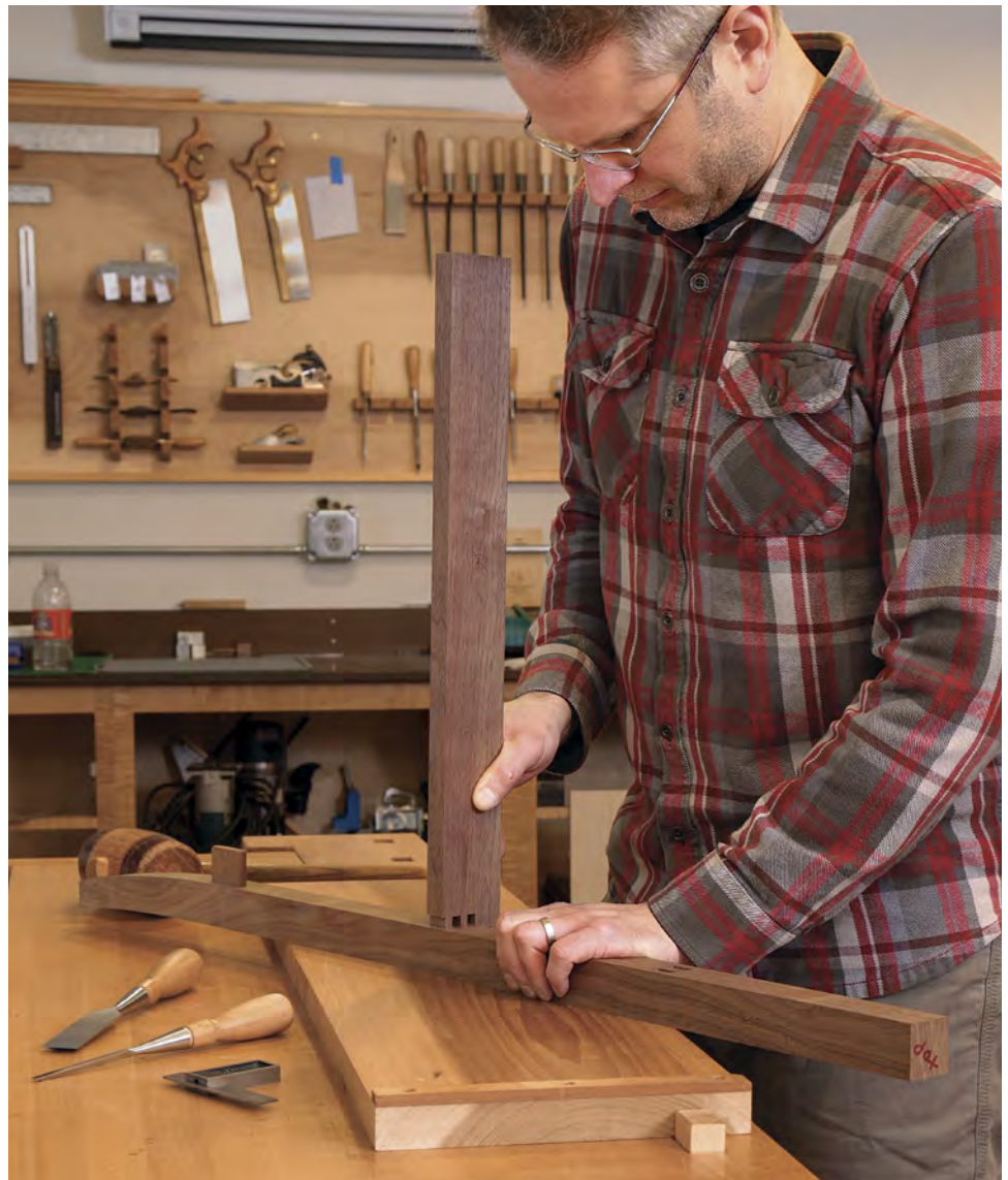
Last task. Square up the rounded corners of the router cuts, removing most of the waste before finishing with a last light paring pass right at the shoulder line.
