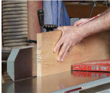
**Square jointer fence means square jointed edge.** Always check for square on the outfeed table a few inches past the blade. If the stock has a bowed edge, place it down for two points of contact.
