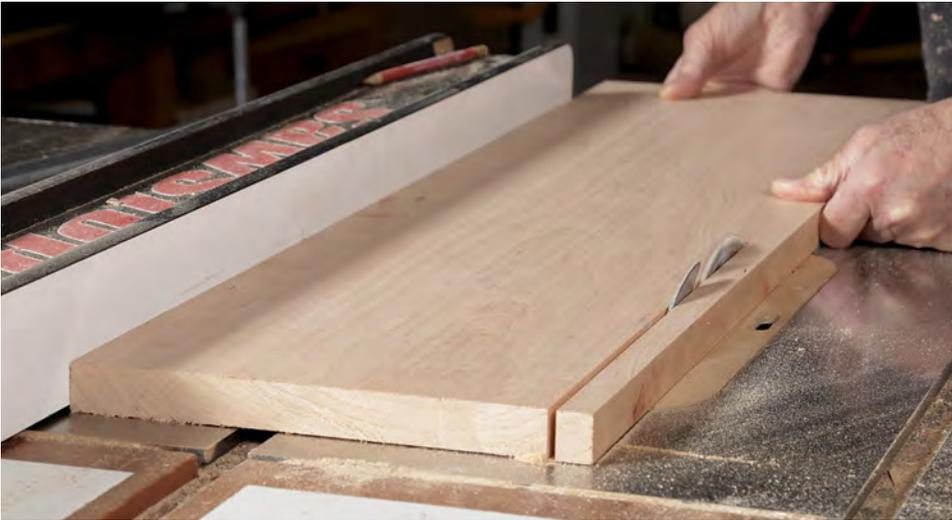
**Rip to width.** Keep the jointed edge against the rip fence; either face can be on the table.
