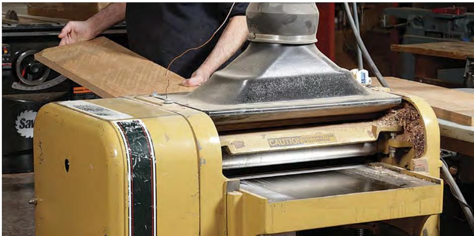
**Plane the second face parallel to the jointed one.** After planing until the second face is completely clean, begin flipping the board end for end between passes to take off an equal amount from each side. Leave the stock  $\frac{1}{8}$  in. too thick.
