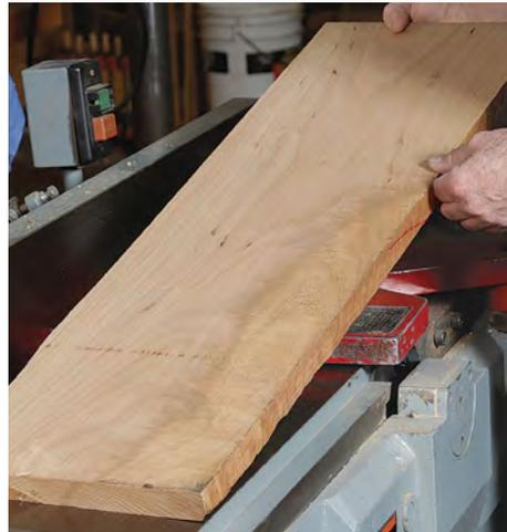
**You don't need a finished surface.** It's sufficient to joint enough wood so the stock will not shift as it goes through the planer.
