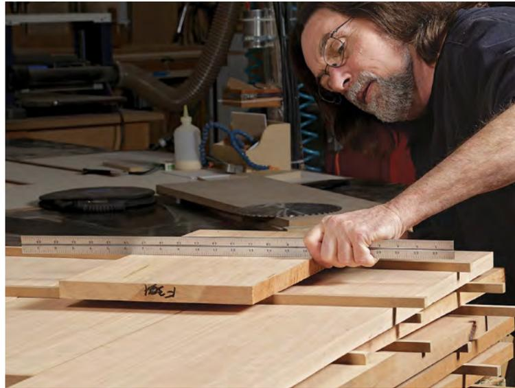
**Watch for cup.** Every few days, check to see how much the boards have cupped. When the board stops cupping, the stock is done moving and is ready for final milling.
