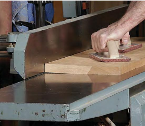
**Pick the correct face to joint.** Typically it's best to place the bowed face down, since it is more stable that way.
