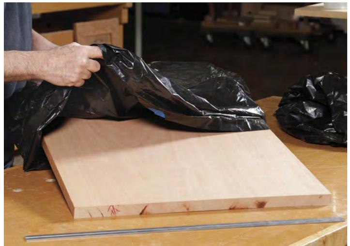
**Plastic bag keeps boards from moving.** Van Dyke uses trash bags for especially wide boards and for longer-term storage.
