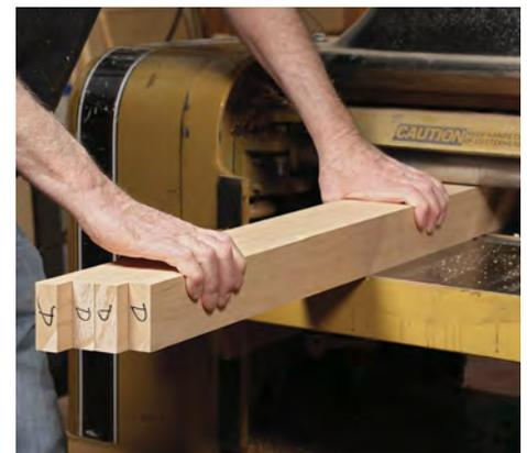
**Edge-plane as a bundle.** Placing their jointed edges down, grip the parts tight as they enter and exit the planer so they act as one board.
