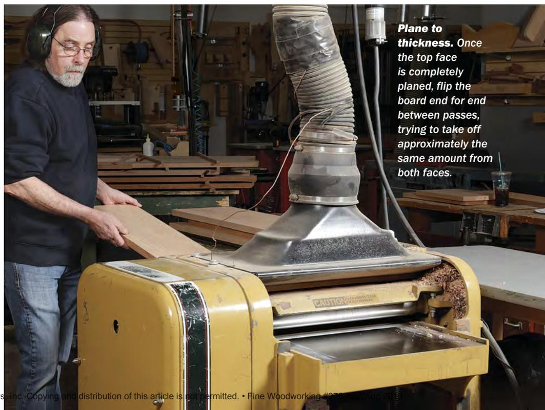
**Plane to thickness.** Once the top face is completely planed, flip the board end for end between passes, trying to take off approximately the same amount from both faces.
