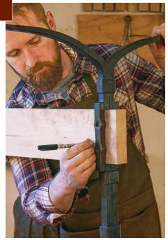
**Steel pattern.** To begin sculpting the joint, Tor Erickson mills a plank to fit the opening in the leg, then traces the outline of the metal.
