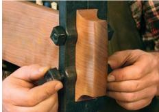
The versatile compression joint. Using nuts and bolts is an extremely strong way to secure the joint, allows for tightening the joint over time, and makes the table simple to disassemble for storage or transport.
