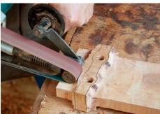
Addition by subtraction. Tor Erickson routs away the waste along both faces of the stretcher, leaving only the areas that will meet metal. He trims to the line and creates a radiused corner using a bandfile belt sander.
