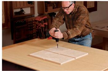
Cut tracks at the tablesaw. Start with a square base and then cut two grooves for the guides. The grooves must be perpendicular to one another. Use a dado set, and cut to final depth in a single pass guided by the rip fence (top). Screw down the jig base (above). Centerlines drawn on the base align with centerlines on the MDF blank for the template.
