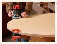
Always rout downhill. Start at the widest point and work toward the end. You can rout two sections with the template above the top (left). Flip the top and template over to rout the other two (below).
