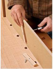
**Guides control the trammel's travel.** They fit into grooves in the base that you'll make next and keep the arm on an elliptical path. Measuring from the bit's cutting edge, locate the first guide half the table's width away, and the second guide half the table's length away (left). Tap T-nuts into the guides, and then bolt the guides to the arm (right).
