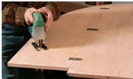
**Trace the template on the real top.** Hand pressure is enough to hold it still at this stage. However, place an X on the template and a matching one on the top so that the template goes back on in the same orientation when it's time to rout. Cut away the waste. Don't leave too much waste—just the pencil line is enough.
