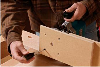
**Glue the router base to the arm.** Because it's made from ½-in. MDF, Gochnour uses a ¼-in. plywood spacer between the base and arm (top). The ¾-in. height equals the thickness of the base that guides the arm's elliptical travel. You'll need longer screws to get through the MDF and still have good purchase in the router's base (above).
