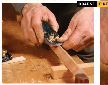
There are many ways to cut a chamfer, but none are as flexible as a block plane. You can cut a straight chamfer, one that tapers in width, and even chamfer around a curve. Do the bulk of the work with the apron plane (above). You might get some tearout, but don't worry. The adjustable-mouth block plane, with its fine shavings, will remove it (right).
