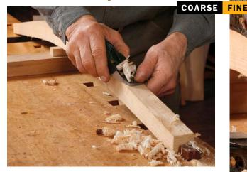
Whether it's been cut at the bandsaw or bent with steam, a curved part needs to be cleaned up and faired to look its best. Set up to remove wood quickly, an apron plane (above) is the perfect tool to get rid of machine marks and the rough grain left behind by steam. It's also a great way to dial in the curve's shape. When it's time to make the last small adjustments to the curve and smooth the part's surface, set down the apron plane and pick up the adjustable-mouth block plane (right).
