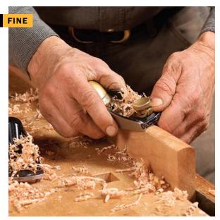
hen you've worked hard to make a table or cabinet, it's a shame to finish it off with a routed edge. A custom edge profile is more suitable for handmade furniture and is no trouble to make. Rough out the shape quickly with the apron plane (left), and then tune its shape and smooth its surface with the adjustable-mouth block plane (above).
