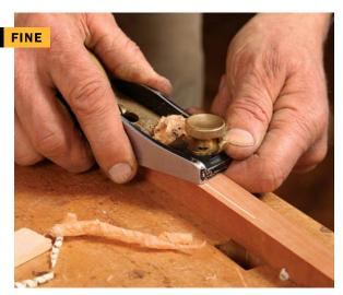
fter gluing a piece of stringing into its groove, quickly work it down near the surrounding surface with the apron plane (left). Speed is what you're after at this stage. Then use the adjustable-mouth block plane to trim the stringing flush with the surface. But don't stop there. Take another pass or two to smooth the inlay and the surrounding wood (above). With its tight mouth and the light shavings, the adjustable-mouth plane can handle even reversing grain and multiple inlay in one area.
