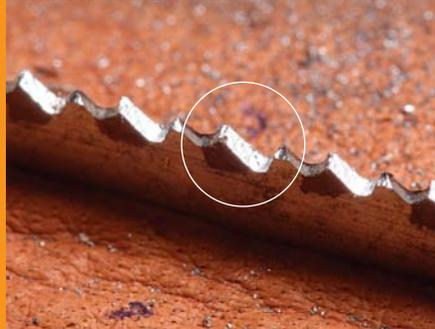
The back of the teeth are easiest to see, so look there for one shiny facet, which means you nailed the angle. Second, since you are filing every other gullet, you need to remove only about half of the tiny flats on the tips of the teeth at this point.
