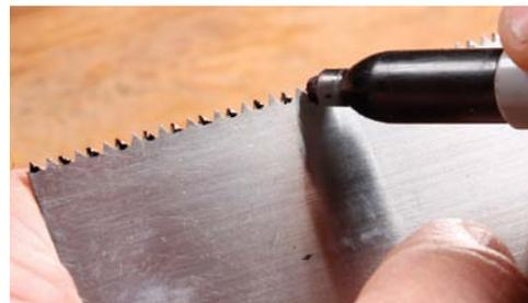
**Mark the teeth now.** Use a marker to dot the teeth that are leaning away from you. Then flip over the saw and do the same on the other side, coloring the remaining teeth.
