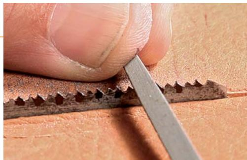
**Wiggle the file into place.** When using the saw file, the goal is to match the sharpening angle that's already there.
