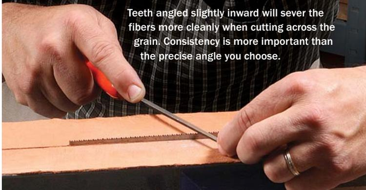
Teeth angled slightly inward will sever the fibers more cleanly when cutting across the grain. Consistency is more important than the precise angle you choose.
