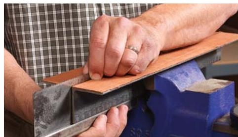
**Clamp the blade.** Most people don't have a traditional saw vise, but you can convert any vise by adding temporary jaws, made from angle-iron lined with leather.
