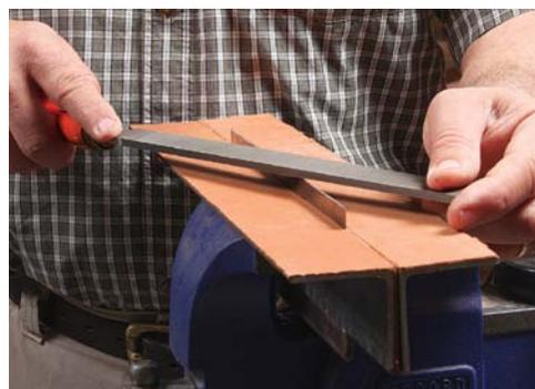
**Joint the teeth.** Filing creates a level reference surface for the rest of the sharpening process. Use a flat, bastard-cut mill file, keeping it level as you push it from heel to toe.
