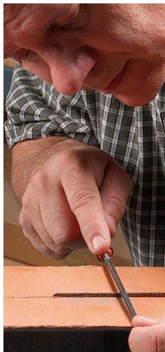
**Light, heavy, light.** Keep the file level as you take two or three light strokes. Then take a look. You should see a nice even facet on the back of the dotted tooth. Then take a more firm stroke, and one last light stroke if needed.
