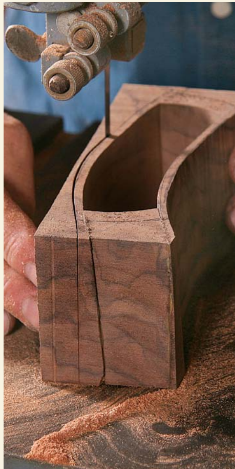
Saw the outside walls. After glue-up, cut the outside walls to free the box from the blank.
