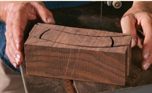
From a blank to a box. With the bandsaw table angled a few degrees, make the two long cuts first, then the short ones to create a four-walled box.
