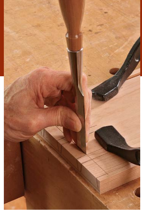
It's familiar at first. Start chiseling half-blind pins as you would through-pins. Place the chisel right in the scribe line (above) and begin with light mallet blows. Then pare out a shallow chip (below). The next mallet blows will be harder and the chips thicker.
