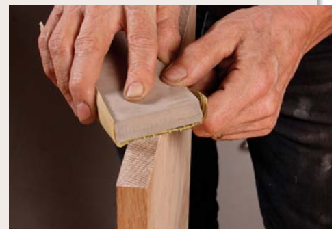
End with the end grain. You can usually stop sanding face grain at 220 grit, but go to 400 grit on end grain for a glass-smooth finish.
