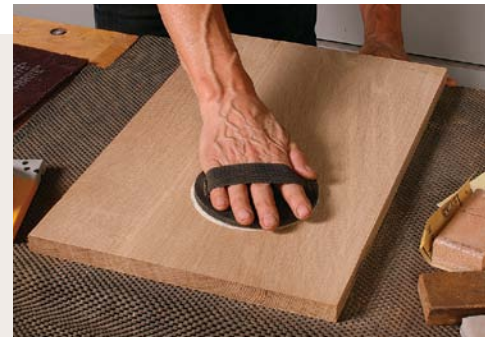
Hand-sanding disks. If you find it tiring to grip a sanding block for long periods, use a strap-on hand pad designed for hook-and-loop disks.
