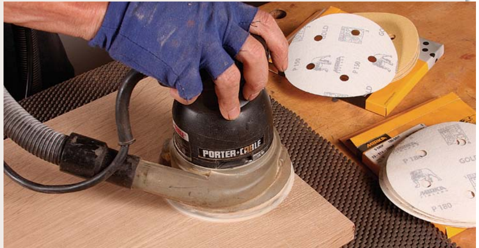
Erase machine marks. Use a 5- or 6-in. random-orbit sander, starting with 150-grit paper and finishing with 180-grit. Jewitt uses cushioned work gloves to dampen the sander's vibration.
