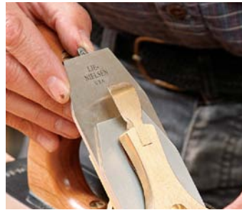
Split adjustments. Planes with Bailey-type adjusters use a wheel to set the blade depth (top) and a lever for lateral changes (bottom).
