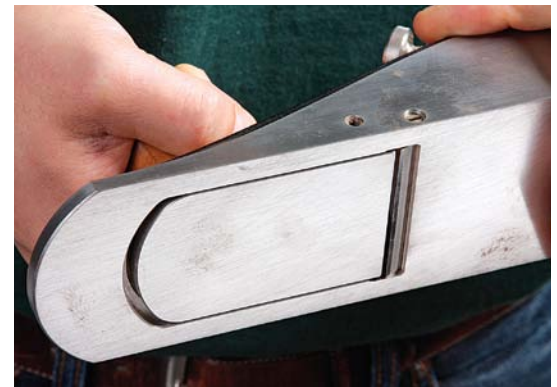
You shouldn't have to remove the blade. Mouth adjustments are made by moving the frog or by sliding a toe, or shoe, at the front of the plane. Planes with a Bedrock-style frog (or similar) let you move the frog with the blade in place by turning screws at the back of the frog. With planes that use a sliding toe to adjust the mouth opening, like the Veritas Custom No. 5, you never have to remove the blade for mouth adjustments.
