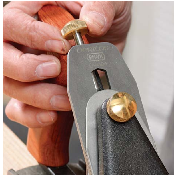
Two in one. Planes with Norris-type adjusters, like the Veritas 5¼ W, combine depth and lateral adjustment into one mechanism. Turning the knob changes the depth and swinging the lever makes lateral adjustments.
